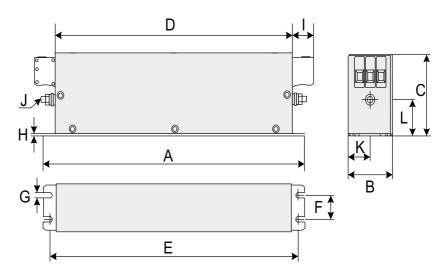
Figure 5-24 Dimensions of FN 3258 series filters (50 A to 180 A)
