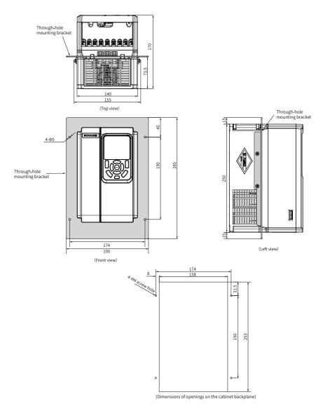
Figure 5-4 MD500-AZJ-A1T3 through-hole mounting bracket and hole dimensions (mm)
