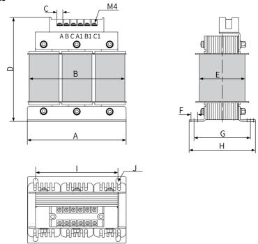
Figure 5-17 Dimensions of AC input reactors (10 A/15 A)
