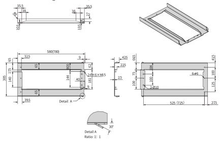
Figure 5-11 Dimensions of the bottom mounting bracket for T10 models
