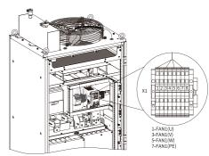
4. Remove the four fixing screws from the top-mounted fan and take out the fan from the AC drive.
