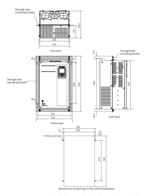
Figure 5-9 MD500-AZJ-A1T8 through-hole mounting bracket and cut-out dimensions (mm)
