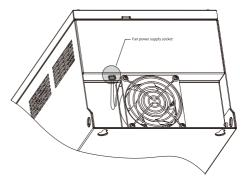
2. Remove the four fixing screws on the fan cover with a screwdriver.
