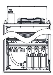
Figure 3-9 Layout of main circuit terminals for T13 models
