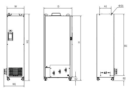
Figure 5-37 Outline and installation dimensions (unit: mm) of MD050NT200G-S to  ${\rm MD050NT400G\text{-}S} \ models$
