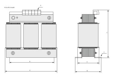
Figure 5-46 Dimensions of output reactors (4-45 A)
