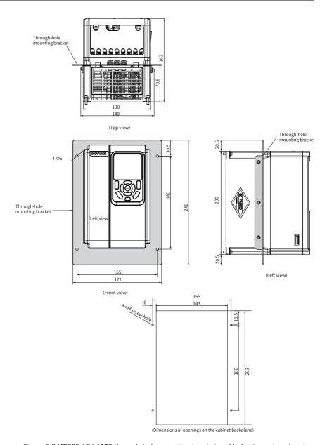
Figure 5-3 MD500-AZJ-A1T2 through-hole mounting bracket and hole dimensions (mm)
