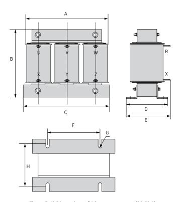
Figure 5-42 Dimensions of AC output reactors (30-60 A)
