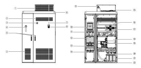
Figure 2-7 Components of the standard cabinet with auxiliary power distribution cabinet
