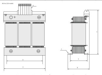
Figure 5-47 Dimensions of output reactors (60–110 A)
