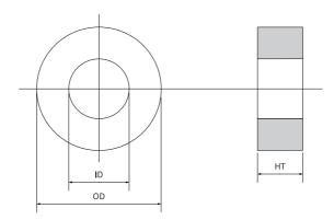
Figure 5-49 Dimensions of the magnetic ring
