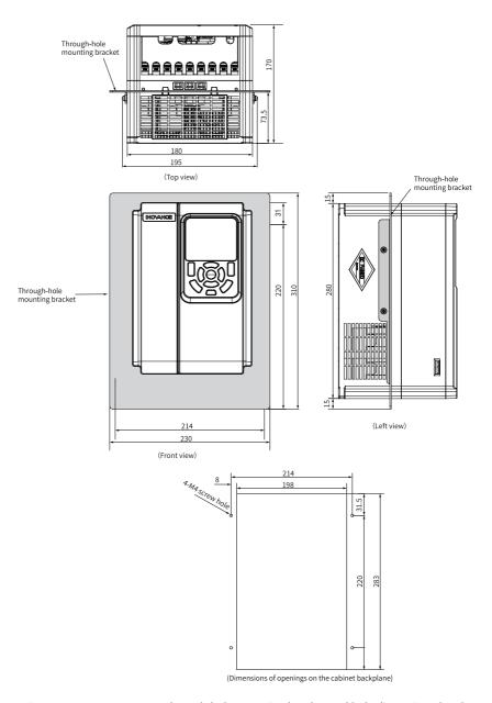
Figure 5-5 MD500-AZJ-A1T4 through-hole mounting bracket and hole dimensions (mm)
