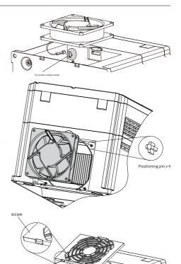
4. After replacing the fan, ensure the fan blows the air upwards.
