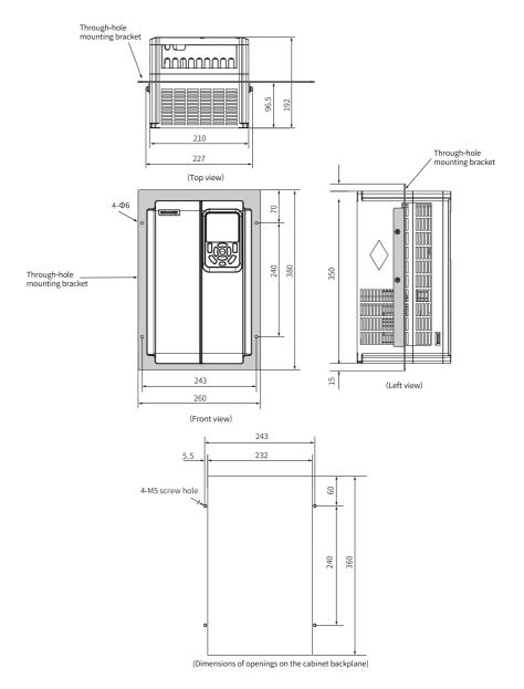
Figure 5-6 MD500-AZJ-A1T5 through-hole mounting bracket and cut-out dimensions (mm)
