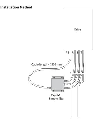
Figure 5-32 Simple filter installation
