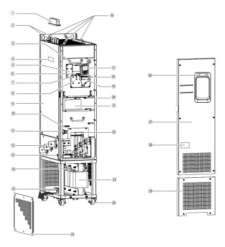
Figure 2-5 Components of T10 to T12 models (with an output AC reactor)
