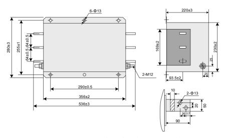
Figure 5-30 Dimensions of Jianli filters (1000 A, unit: mm)
