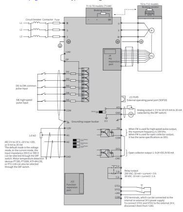
Figure 3-2 Standard wiring diagram (T1 to T12)
