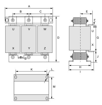
Figure 5-45 Dimensions of AC output reactors (330 A)
