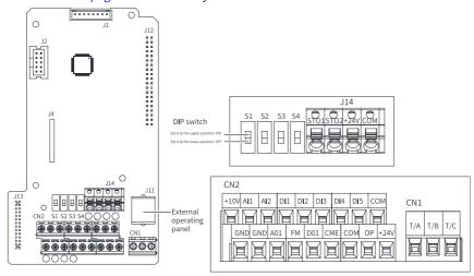
Figure 3-10 Layout of control circuit terminals
