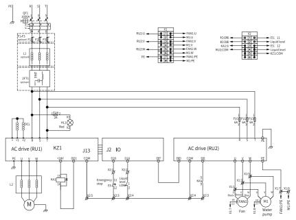
Figure 3-3 Electrical connection in the cabinet (T13)
