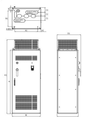
Figure 4-6 Outline dimensions and mounting dimensions of T13 models (without auxiliary power distribution cabinet)
