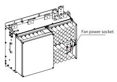
Remove the four fixing screws from the fan and take out the fan from the AC drive. Note that the fan direction is from right to left.
