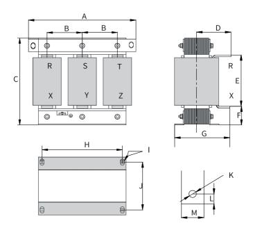
Figure 5-21 Dimensions of AC input reactors (150-330 A)
