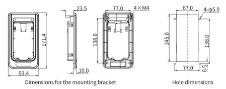
Figure 5-52 Base mounting bracket dimensions and hole sizes (mm) of the MDKE-10
