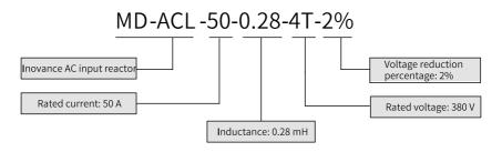
Figure 5-16 AC input reactor model
