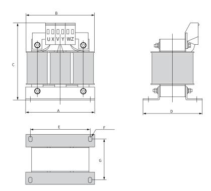
Figure 5-39 Dimensions of AC output reactors (5-10 A)
