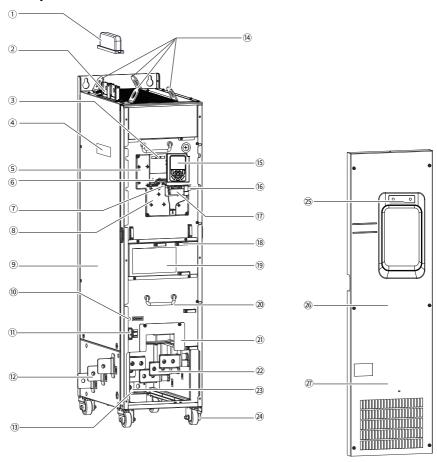
Figure 2-4 Components of T10 to T12 models (without an output AC reactor)
