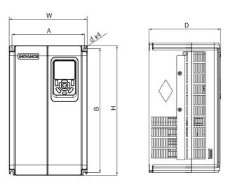
Figure 4-2 Outline dimensions and mounting dimensions of T5 to T6 models
