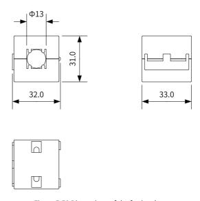
Figure 5-50 Dimensions of the ferrite clamp
