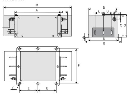
Figure 5-26 Dimensions of FN 3359 series filters (320 A to 2500 A)
