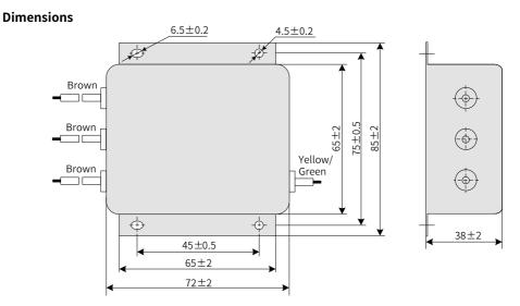
Figure 5-31 Outline dimensions of the simple filter
