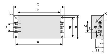
Figure 5-28 Dimensions of Jianli filters (50-200 A)
