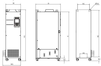
Figure 4-4 Outline dimensions and mounting dimensions of T10 to T12 models (without AC output reactor)
