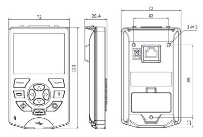
Figure 5-53 Dimensions of the SOP-20-810 (unit: mm)
