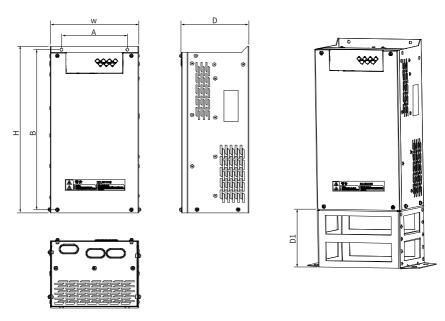
Figure 5-35 Outline dimensions of MD050 series AFE unit (unit: mm)
