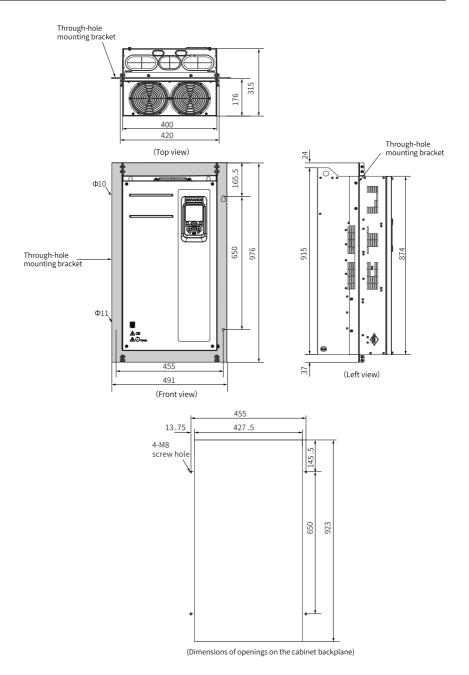
Figure 5-10 MD500-AZJ-A1T9 through-hole mounting bracket and cut-out dimensions (mm)
