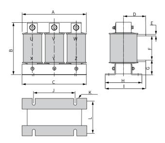
Figure 5-43 Dimensions of AC output reactors (80-120 A)
