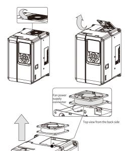
2. Pull the fan upwards and unplug the power cable connector from the socket.
