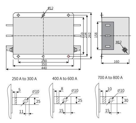
Figure 5-29 Dimensions of Jianli filters (250-800 A, unit: mm)
