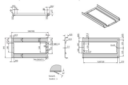
Figure 5-13 Dimensions of the bottom mounting bracket for T12 models
