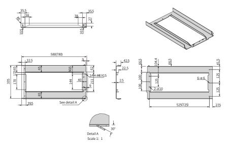
Figure 5-12 Dimensions of the bottom mounting bracket for T11 models
