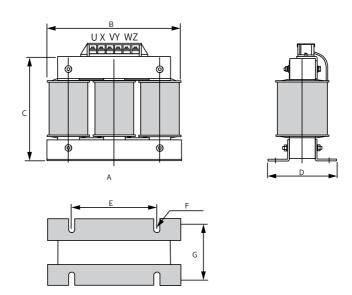
Figure 5-41 Dimensions of AC output reactors (20 A)
