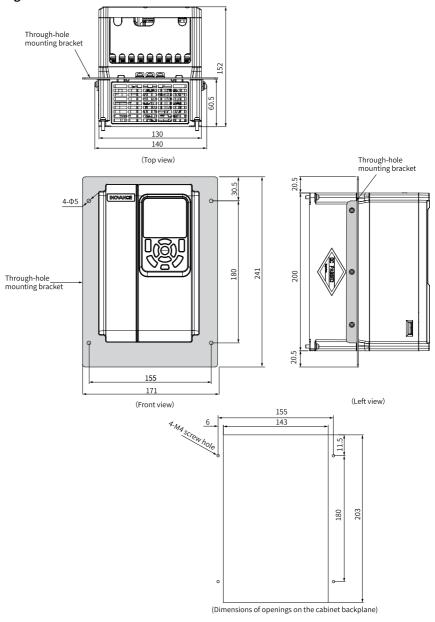
Figure 5-2 MD500-AZJ-A1T1 through-hole mounting bracket and hole dimensions (mm)
