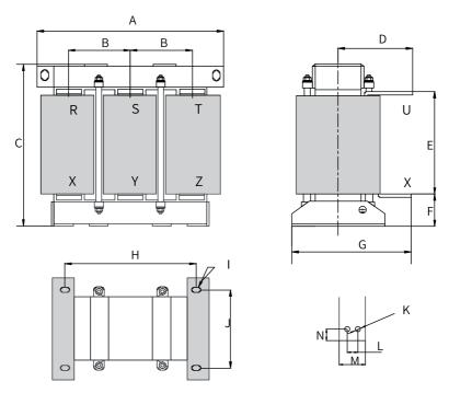
Figure 5-23 Dimensions of AC input reactors (800 A/1000 A)
