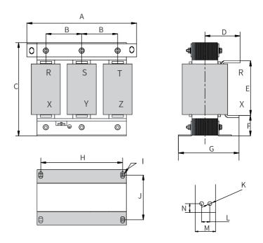
Figure 5-22 Dimensions of AC input reactors (490 A/660 A)
