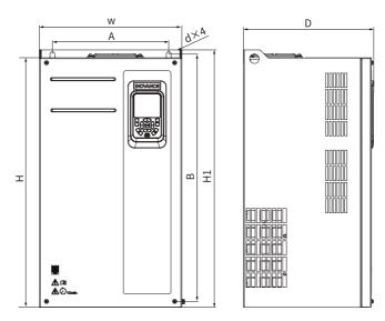
Figure 4-3 Outline dimensions and mounting dimensions of T7 to T9 models
