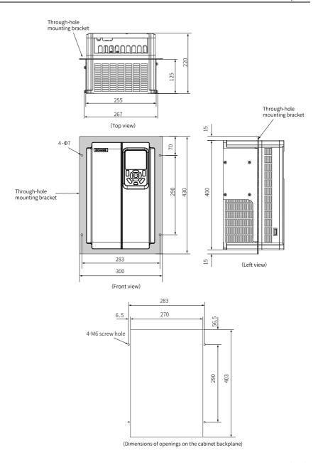
Figure 5-7 MD500-AZJ-A1T6 through-hole mounting bracket and cut-out dimensions (mm)
