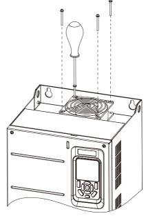
3. Remove the fan and fan cover from the drive.
