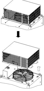
2. Remove the baffle plate as shown in the figure.
