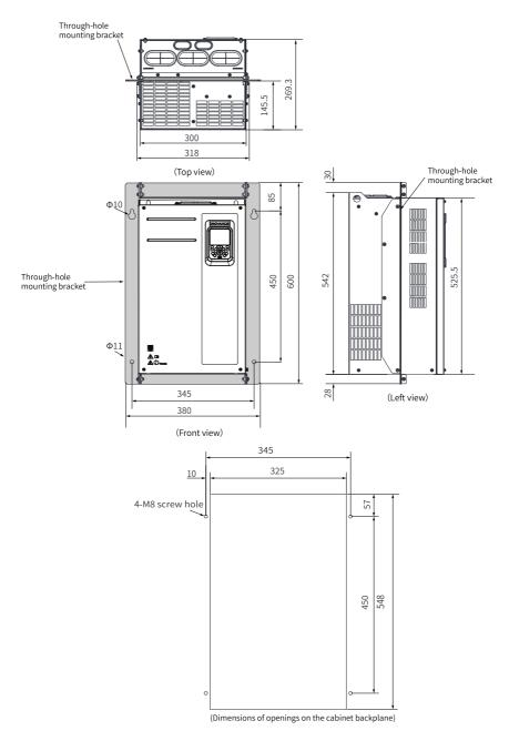
Figure 5-8 MD500-AZJ-A1T7 through-hole mounting bracket and cut-out dimensions (mm)
