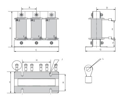
Figure 5-19 Dimensions of 50 A (0.28 mH)/60 A AC input reactors
