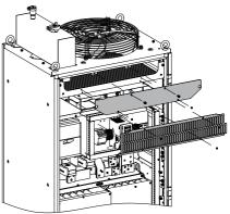
Disconnect the cables connecting the X1 terminal block to the top-mounted fan and pull out the cables from the wiring tray. Remove cables of terminals 1, 3, 5, and 7 only.
