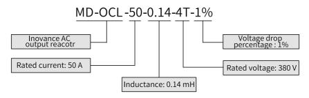
Figure 5-38 AC output reactor model
