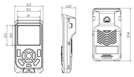
Figure 5-51 Dimensions of the MDKE-10 (unit: mm)
