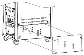
3. Remove the six screws on the drive, install the copper busbars, and then fasten the six screws.
