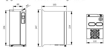
Figure 5-33 Dimensions of MDBUN series braking units (MDBUN-45-2T to MDBUN-90-2T;
