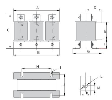
Figure 5-20 Dimensions of AC input reactors (80-120 A)
