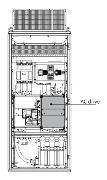
2. Remove baffle plates A and B in sequence from the AC drive.
