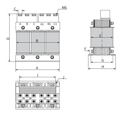
Figure 5-18 Dimensions of 40 A/50 A (1.2 mH) AC input reactors
