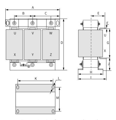
Figure 5-44 Dimensions of AC output reactors (150-250 A)
