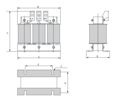
Figure 5-40 Dimensions of AC output reactors (15 A)
