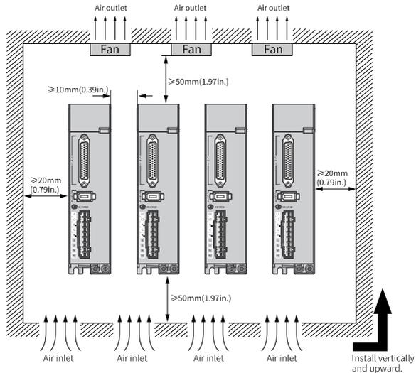
Figure 1-3 Clearance for side-by-side installation
