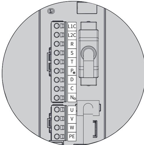
Figure 4-11 Main circuit terminal pin layout of servo drives in size C (SV660PT3R5I, SV660PT5R4I) and size D (SV660PT8R4I, SV660PT012I)
