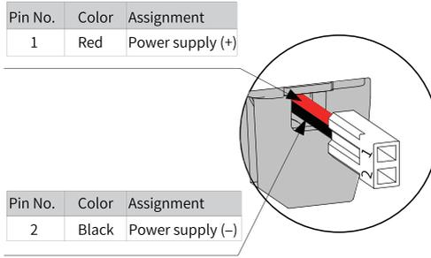
Figure 4-37 Lead wire color of the battery box
