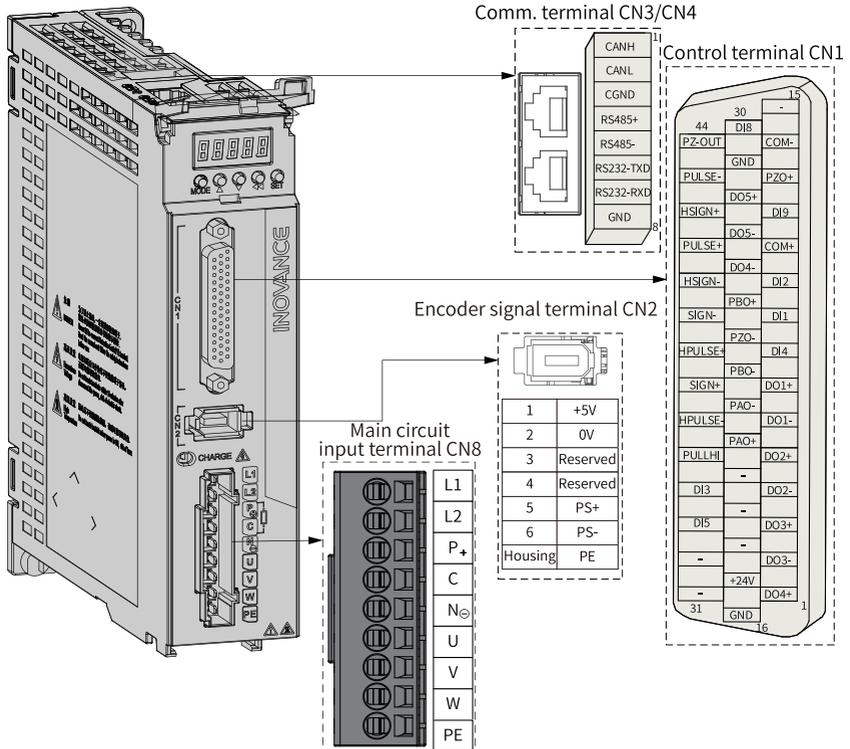
Figure 4-1 Terminal pin layout of servo drives in size A
