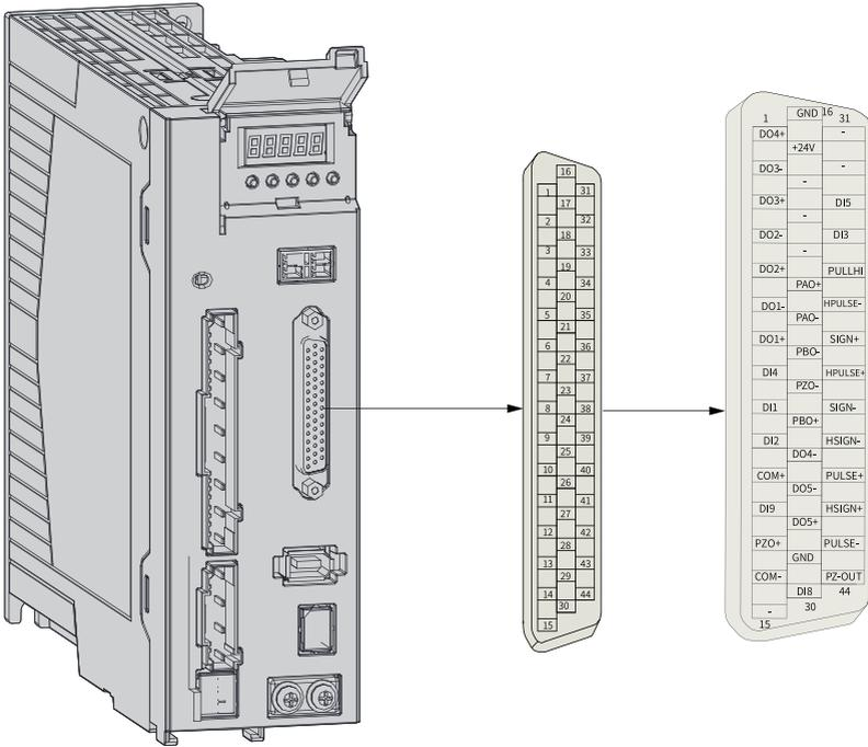
Figure 4-23 Control terminal pin layout of servo drives in sizes C, D, and E
