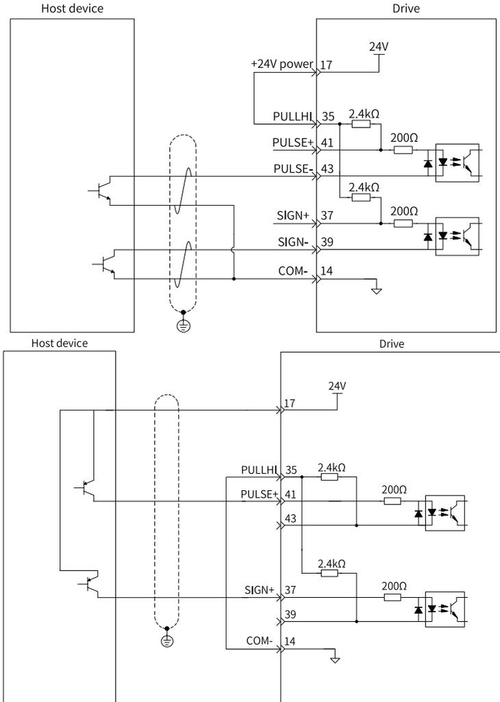
Figure 4-24 Correct: The internal 24 V power supply of the servo drive is used.
