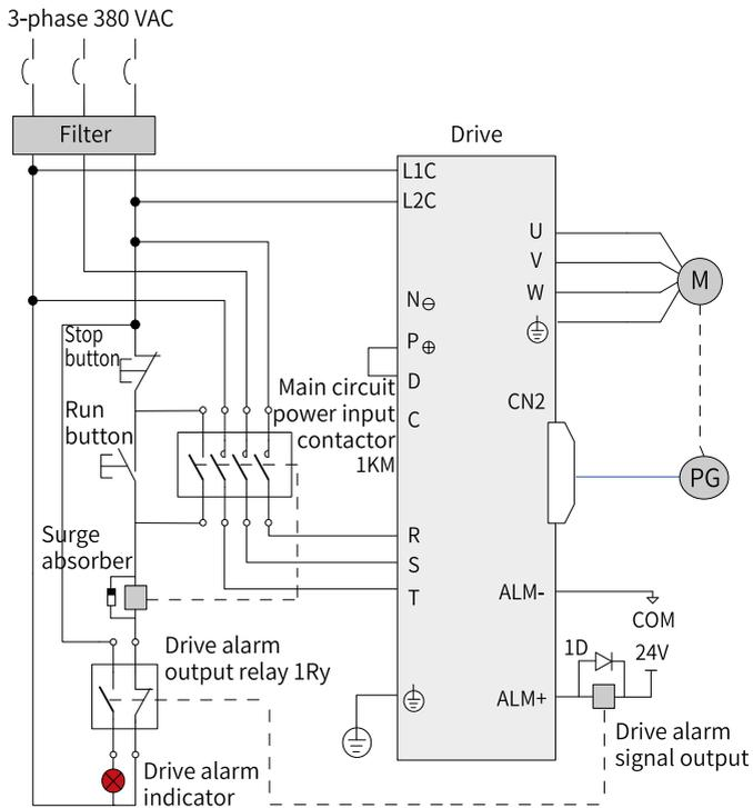
Figure 4-19 Main circuit wiring of three-phase 380 V models
