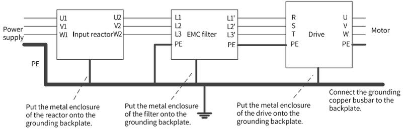
Figure 1-12 Installing the AC input reactor
