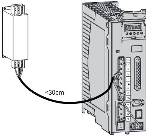
Figure 1-13 Installing the AC input reactor
