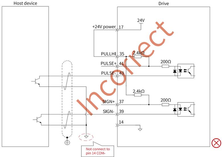
Figure 4-25 Incorrect: Pin 14 (COM-) is not connected, leading to failure in forming a closed-loop circuit.
