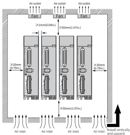
Figure 1-4 Clearance for compact installation
