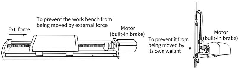
Figure 4-33 Application of the brake
