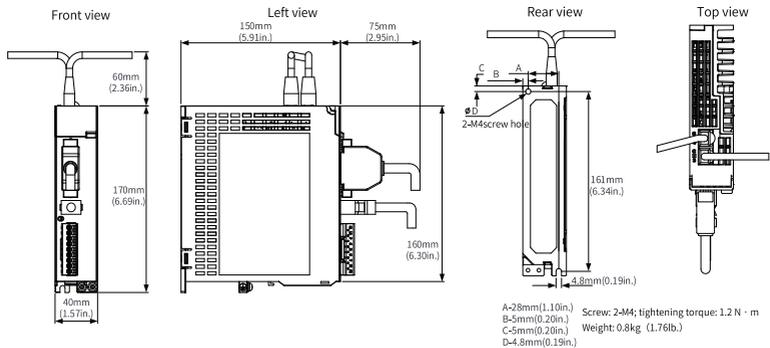
Figure 1-6 Dimension drawing of servo drives in size A
