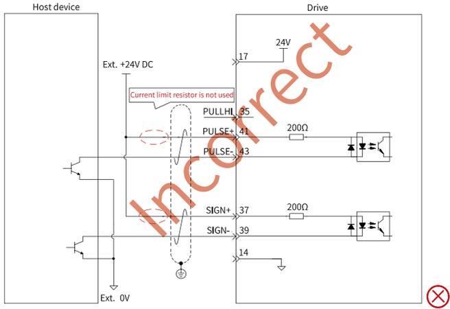
Figure 4-26 Incorrect wiring example 1: The current limiting resistor is not connected, resulting in terminal burnout.
