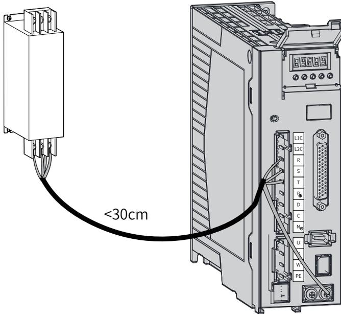
Figure 4-16 Installing the filter
