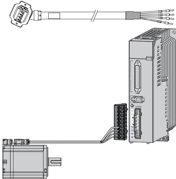
Figure 4-14 Wiring between the servo drive and terminal-type motor
