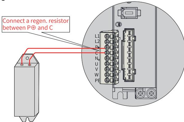
Figure 4-50 Wiring of external regenerative resistor
