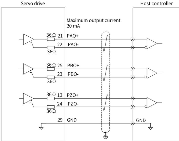
Figure 4-31 Differential receiving circuit
