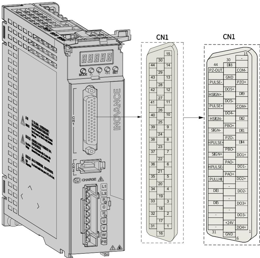
Figure 4-22 Control terminal pin layout of servo drives in sizes A and B
