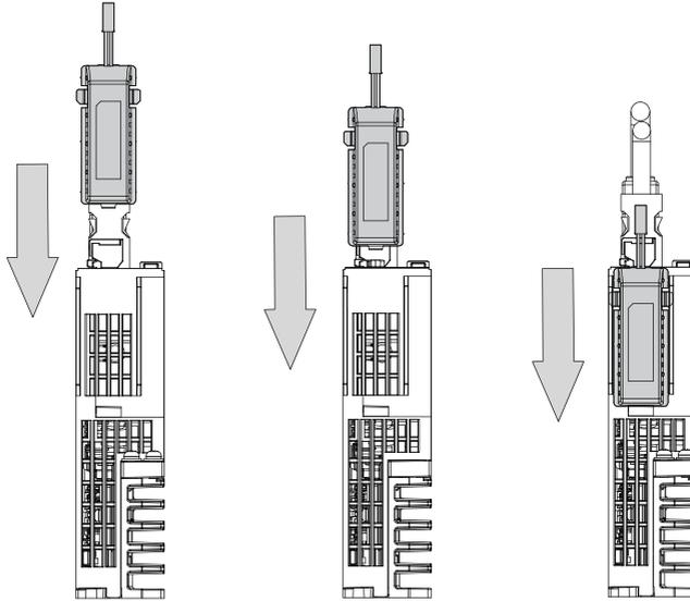
Figure 4-38 Installing the battery box (bottom view)
