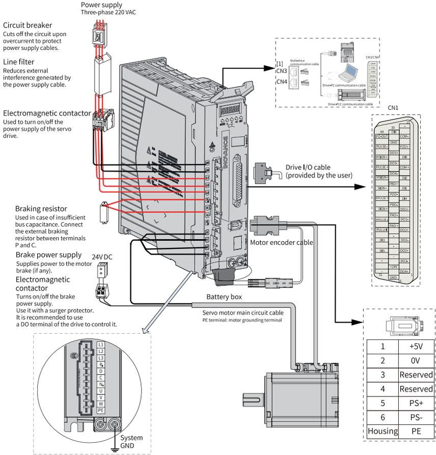
Figure 2-2 Wiring example of a three-phase 220V system
