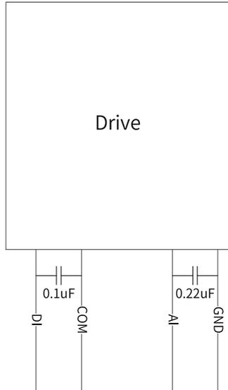
Figure 7-2 I/O signal cables with capacitance increased
