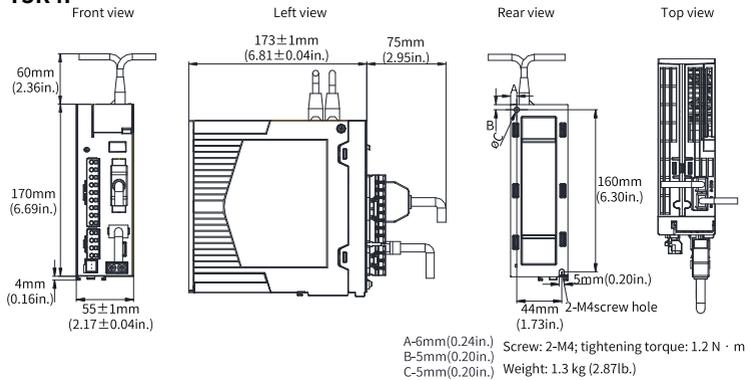
Figure 1-8 Dimension drawing of servo drives in size C
