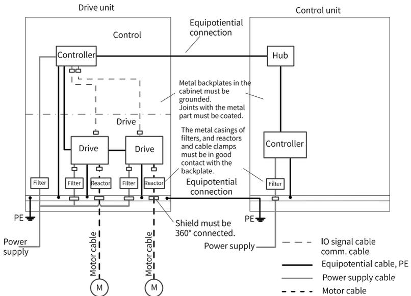
Figure 4-20 Recommended wiring for the control cabinet system
