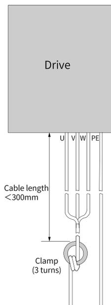
Figure 1-14 Installation of the magnetic ring
