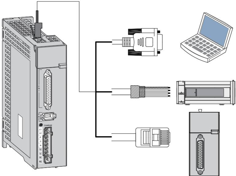
Figure 4-40 Wiring of communication cables
