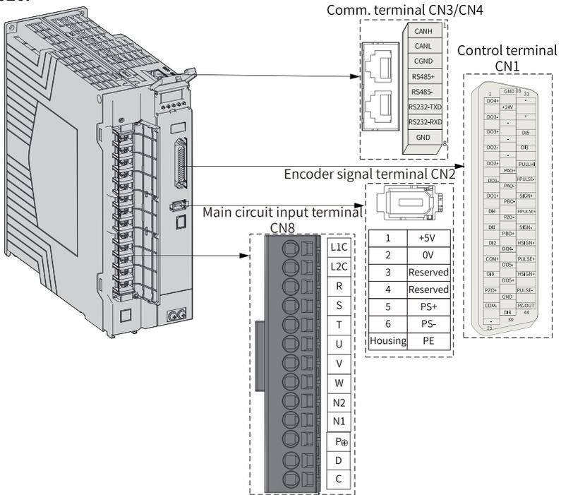
Figure 4-5 Terminal pin layout of servo drives in size E
