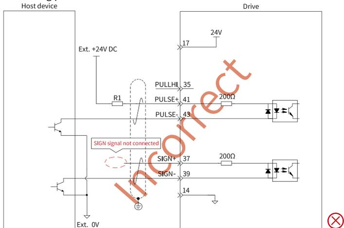
Figure 4-28 Incorrect wiring example 3: The SIGN port is not connected, preventing these two ports from receiving pulses.
