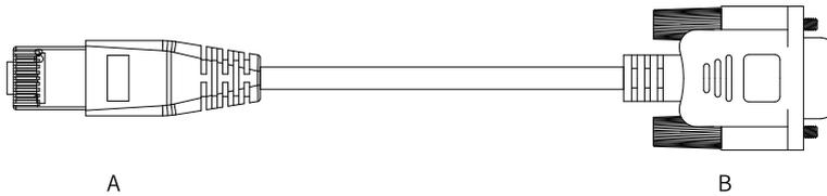
Figure 4-48 PC communication cable
