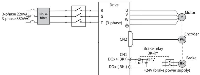
Figure 4-34 Wiring of the brake
