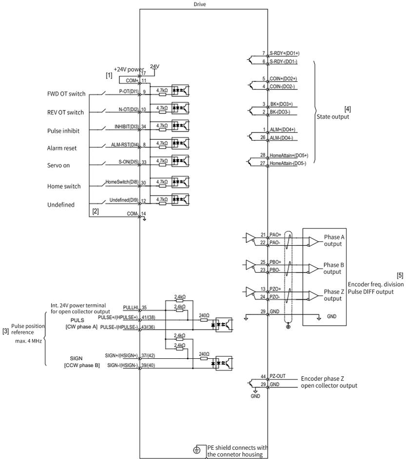
Figure 3-1 Wiring diagram of the Position Control Mode
