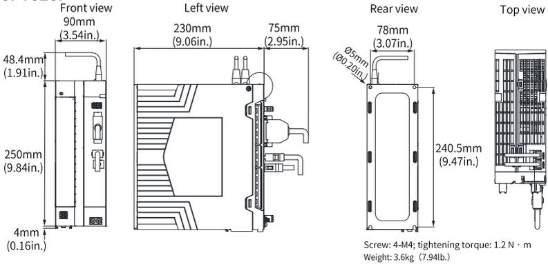
Figure 1-10 Dimension drawing of servo drives in size E
