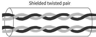
Figure 4-21 Diagram of shielded twisted pairs
