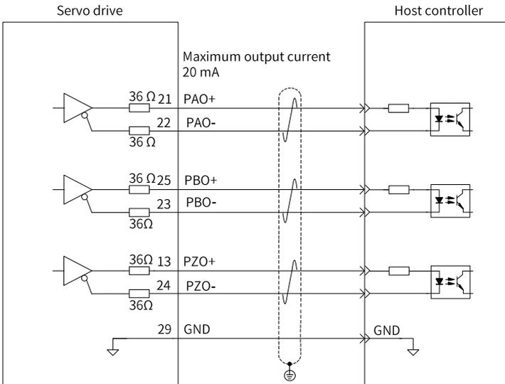
Figure 4-32 Optocoupler receiving circuit
