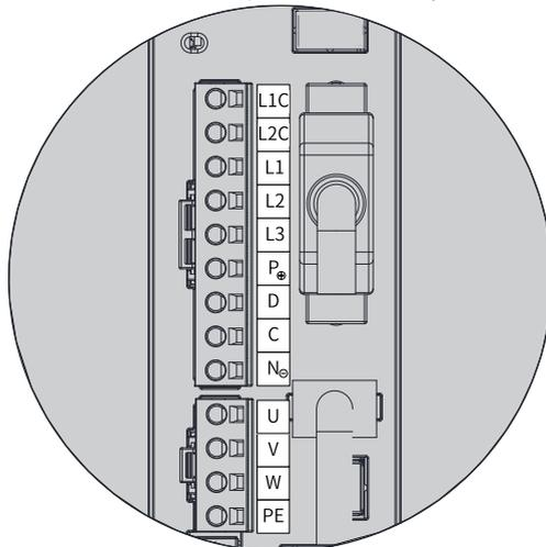
Figure 4-10 Main circuit terminal pin layout of servo drives in size C (SV660PS7R6I) and size D (SV660PS012I)
