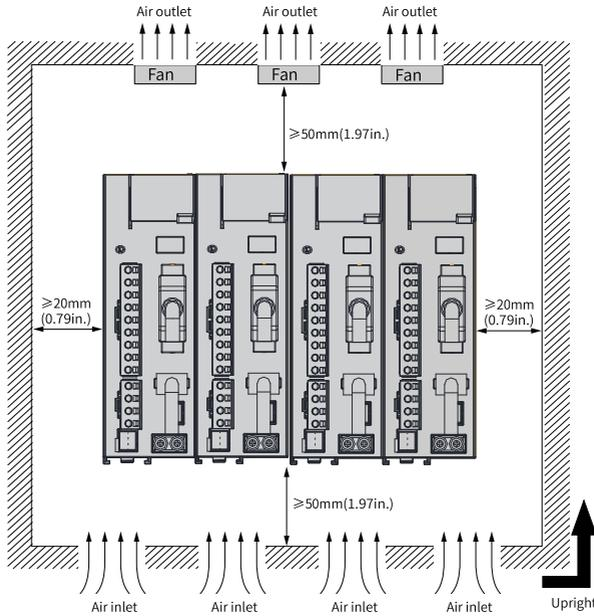
Figure 1-5 Zero-clearance installation
