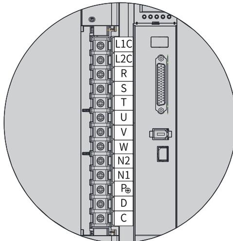
Figure 4-12 Pin assignment of main circuit terminal of servo drives in size E
