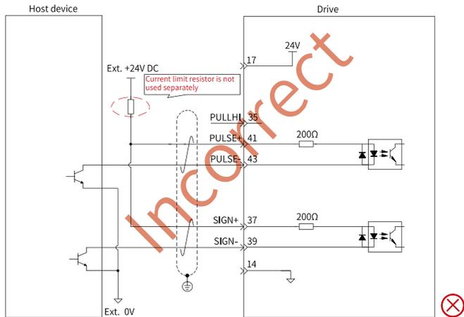
Figure 4-27 Incorrect wiring example 2: Multiple terminals share the same current limiting resistor, resulting in pulse receiving error.
