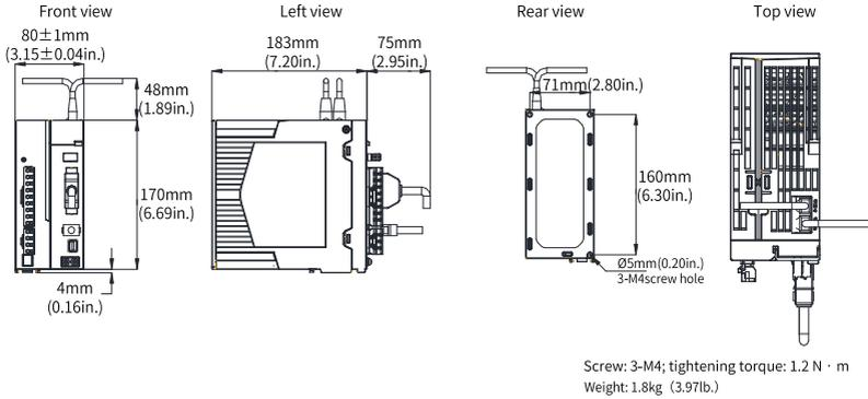
Figure 1-9 Dimension drawing of servo drives in size D
