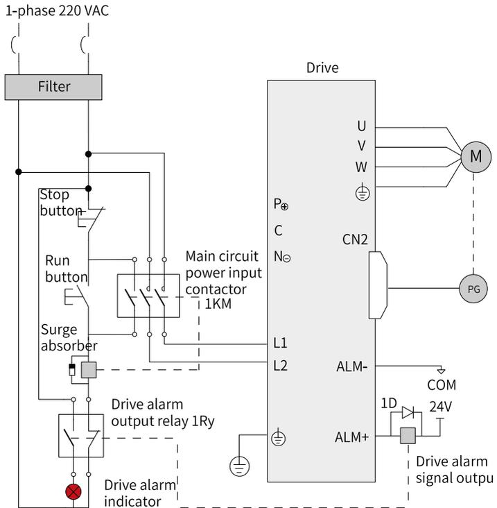
Figure 4-17 Main circuit wiring
