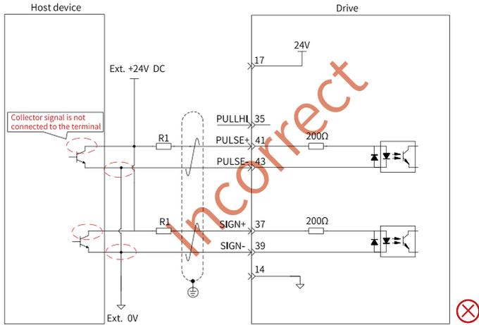
Figure 4-29 Incorrect wiring example 4: Terminals are connected incorrectly, resulting in terminal burnout.
