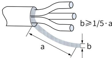
Figure 4-13 Lead-out of the motor cable shield
