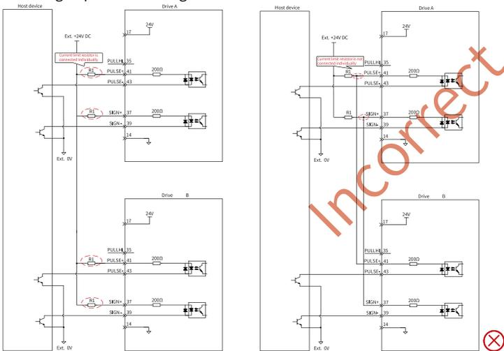
Figure 4-30 Incorrect wiring example 5: Multiple terminals share one current limiting resistor, resulting in a pulse receiving error.
