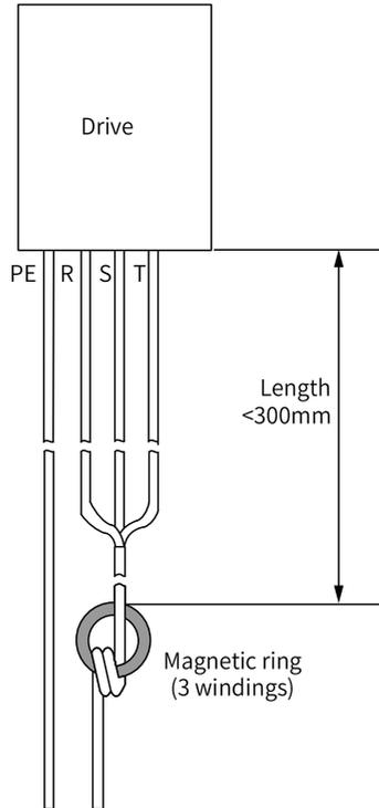
Figure 7-1 Magnetic ring on the input side
