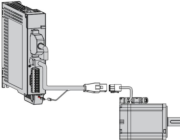
Figure 4-36 Signal wiring example of the absolute encoder<sup>[1]</sup>
