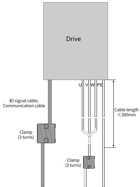
Figure 1-15 Installation of the ferrite clamp
