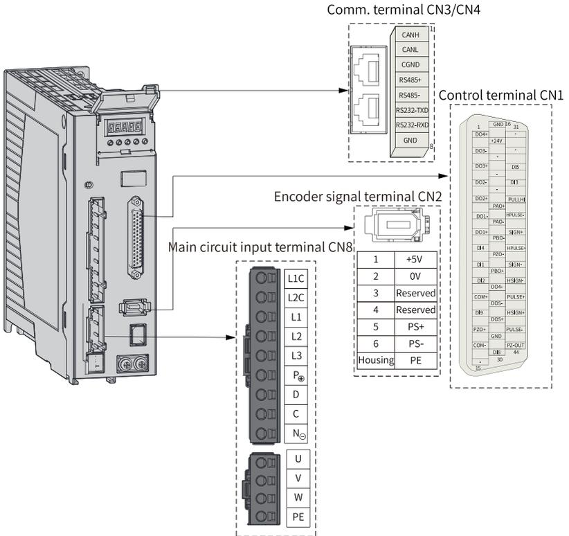
Figure 4-3 Terminal pin layout of servo drives in size C (SV660PS7R6I) and size D (SV660PS012I)
