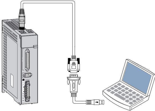
Figure 4-49 PC communication cable
