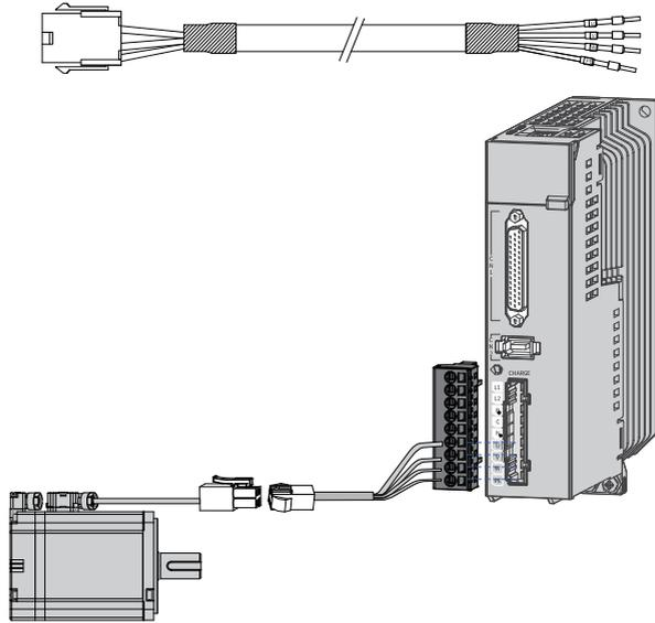
Figure 4-15 Wiring between the servo drive and terminal-type motor
