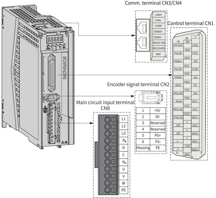
Figure 4-2 Terminal pin layout of servo drives in size B
