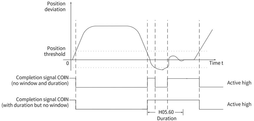
Figure 2-24 Schematic diagram for the window time (H05.59) and hold time (H05.60) of positioning completed signal
