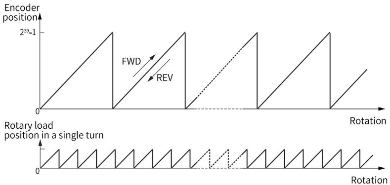
Figure 2-84 Relation between encoder feedback position and the single-turn position of the rotating load
