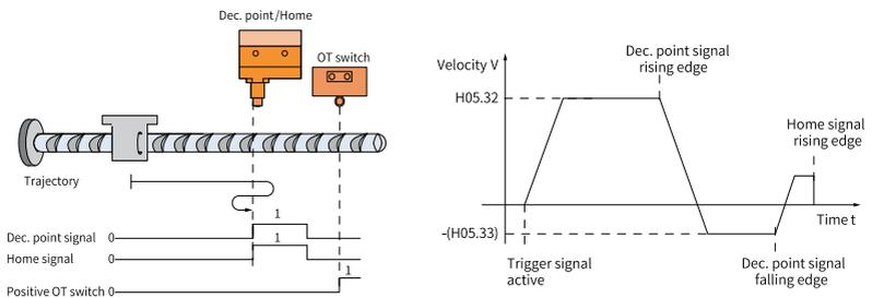
Figure 2-27 Motor running curve and speed in mode 0
