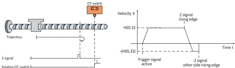
Figure 2-30 Motor running curve and speed in mode 2
