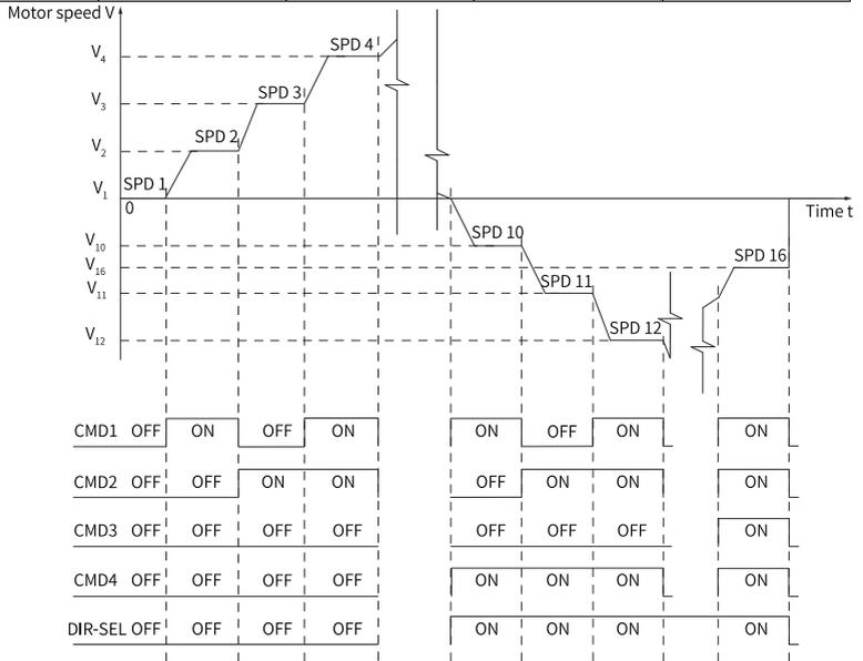
Figure 2-54 Example of multi-speed curve
