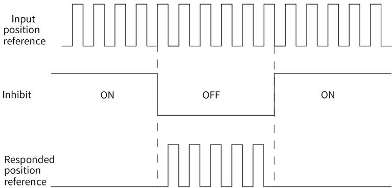
Figure 2-13 Waveform example for position reference inhibited
