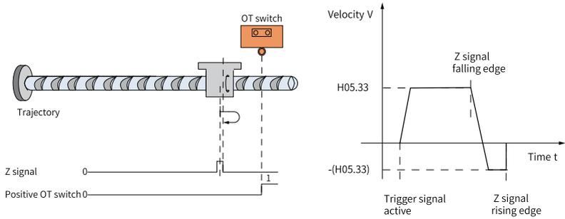
Figure 2-31 Motor running curve and speed in mode 2
