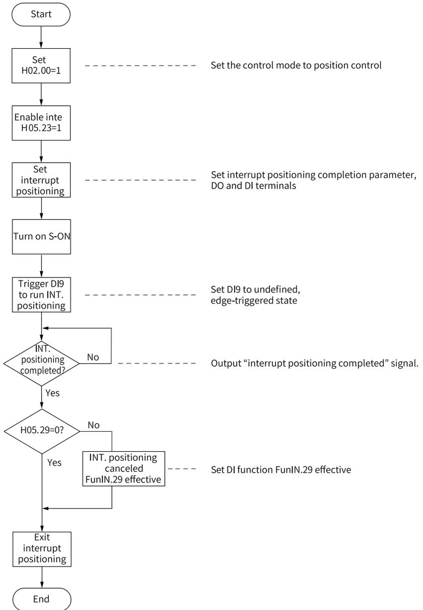
Figure 2-25 Flowchart of interrupt positioning signal
