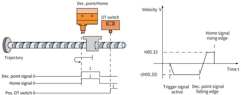
Figure 2-28 Motor running curve and speed in mode 0
