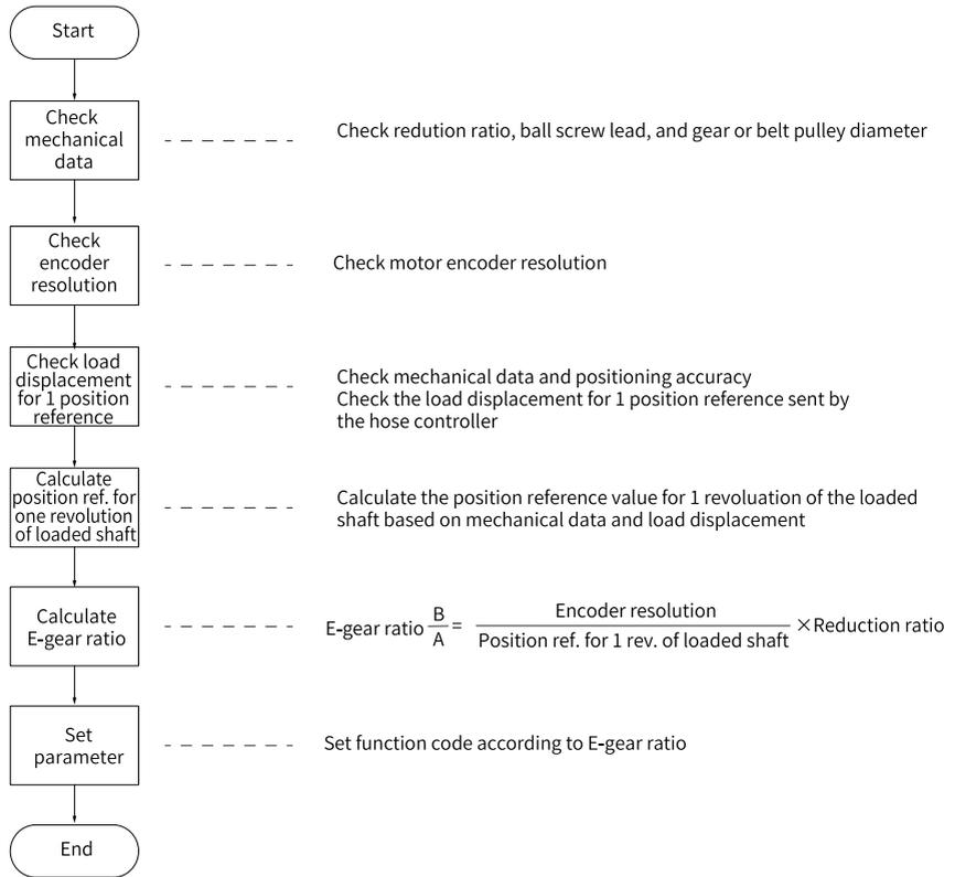
Figure 2-15 Procedure for setting the electronic gear ratio
