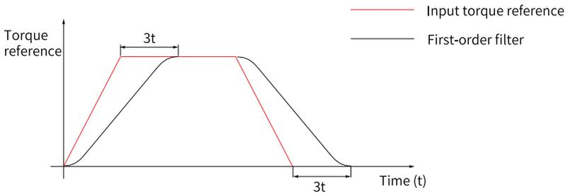
Figure 2-69 First-order filter for trapezoid torque references
