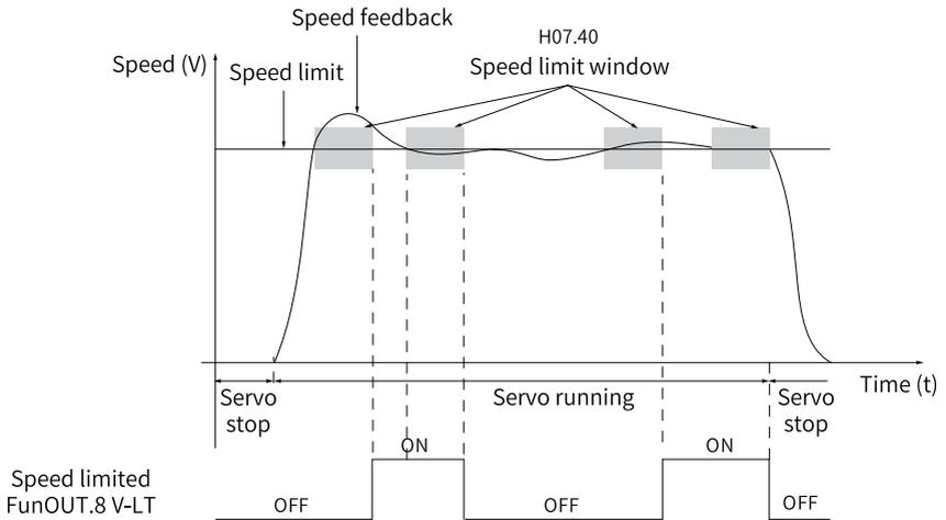
Figure 2-78 Example of speed limit DO waveform
