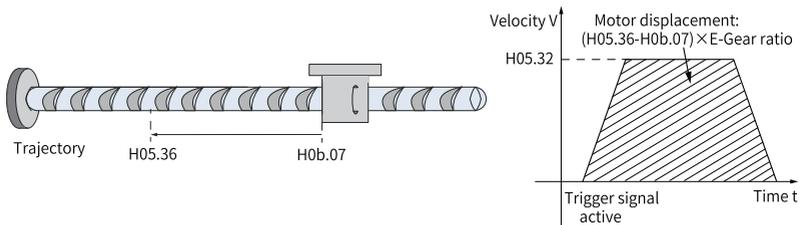
Figure 2-43 Motor running curve and speed in mode 15
