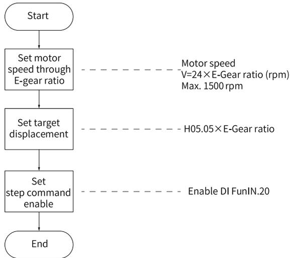
Figure 2-8 Flowchart for setting step reference as the position reference source
