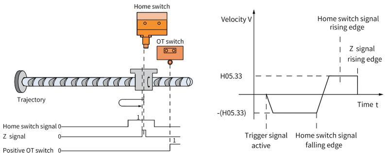
Figure 2-34 Motor running curve and speed in mode 4
