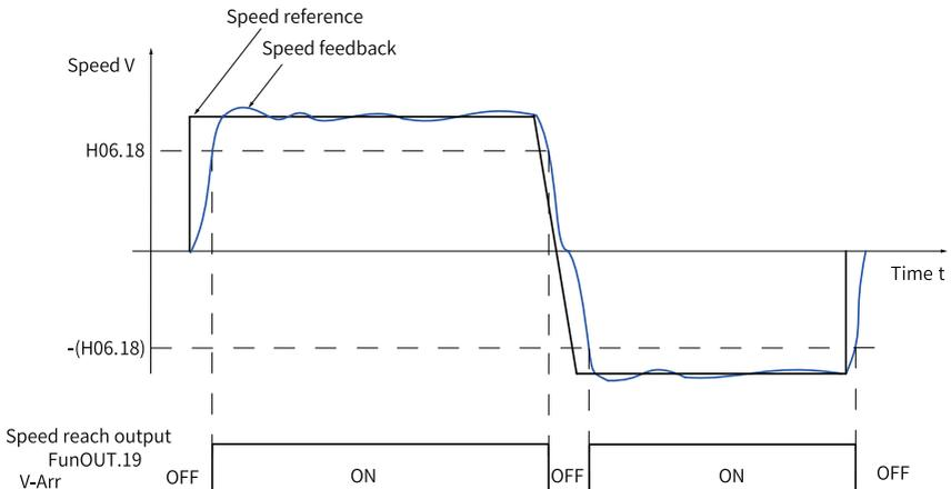
Figure 2-61 Waveform of the speed reach (V-Arr) signal
