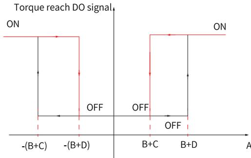
Figure 2-80 Description of torque reach output
