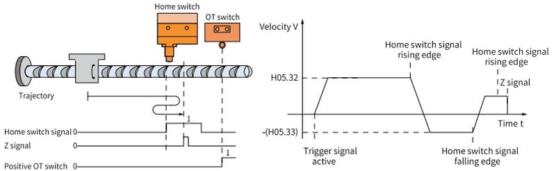
Figure 2-33 Motor running curve and speed in mode 4
