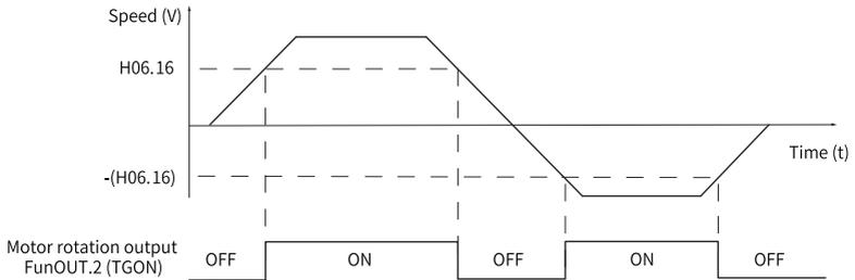
Figure 2-59 Waveform of motor rotation (TGON) signal
