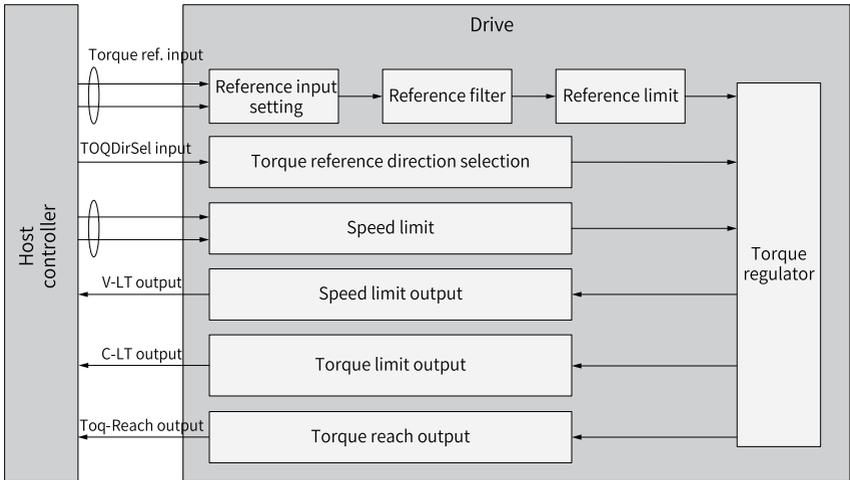
Figure 2-64 Signal exchange between the drive and the host controller
