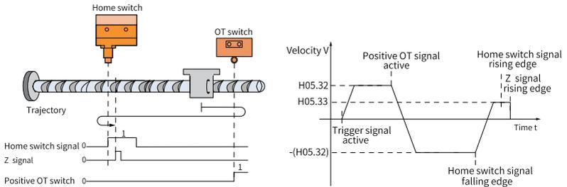
Figure 2-35 Motor running curve and speed in mode 4
