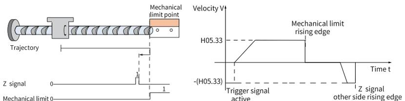
Figure 2-41 Motor running curve and speed in mode 12
