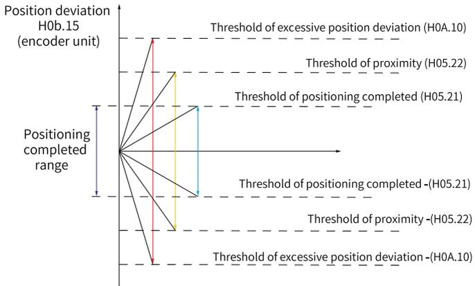
Figure 2-23 Signals related to position deviation
