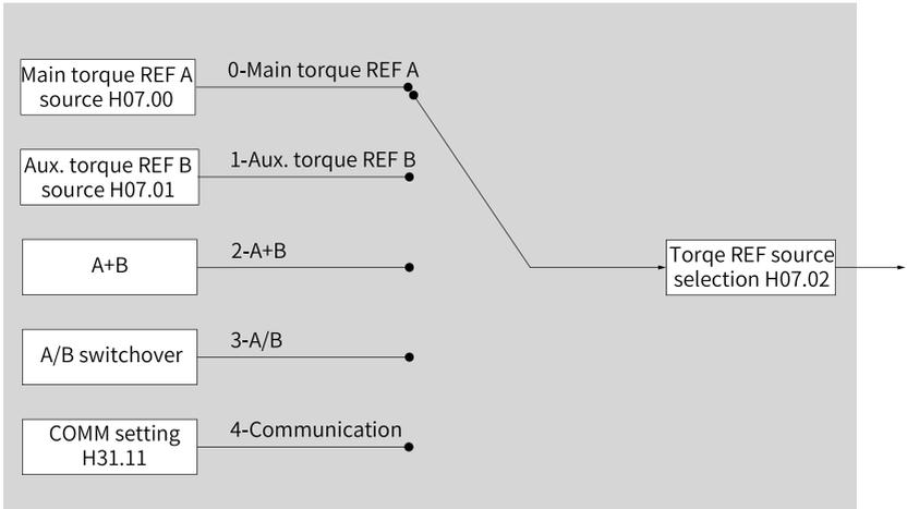
Figure 2-66 Torque reference sources
