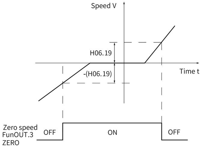
Figure 2-62 Waveform of the zero speed (V-Zero) signal
