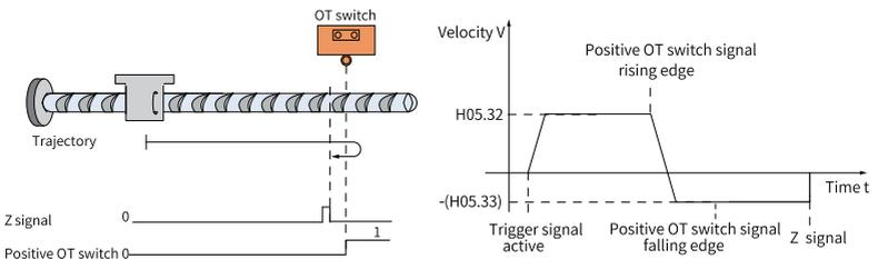
Figure 2-38 Motor running curve and speed in mode 8
