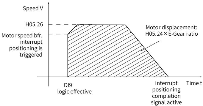
Figure 2-26 Motor operating curve during interrupt positioning
