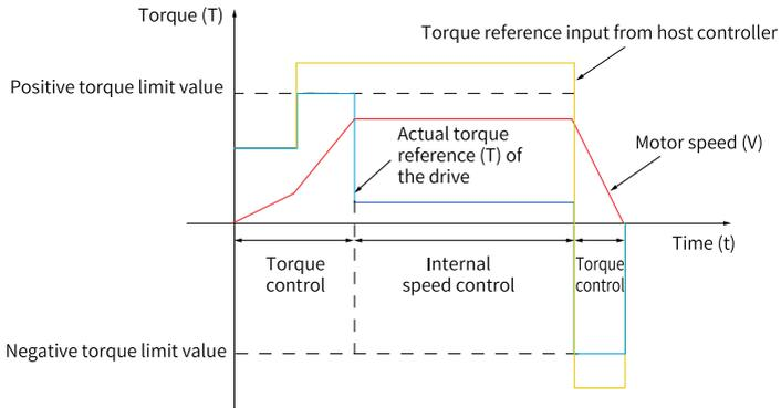
Figure 2-70 Torque reference and torque limit
