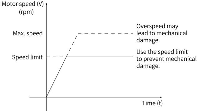
Figure 2-75 Speed limit in the torque control mode
