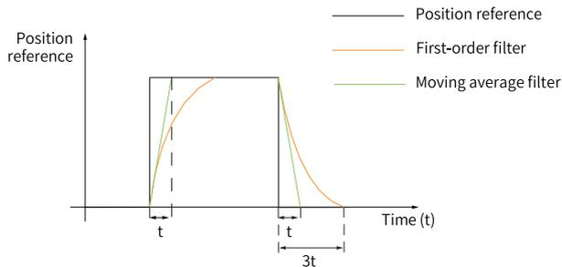
Figure 2-19 First-order filter and moving average filter for rectangular position references
