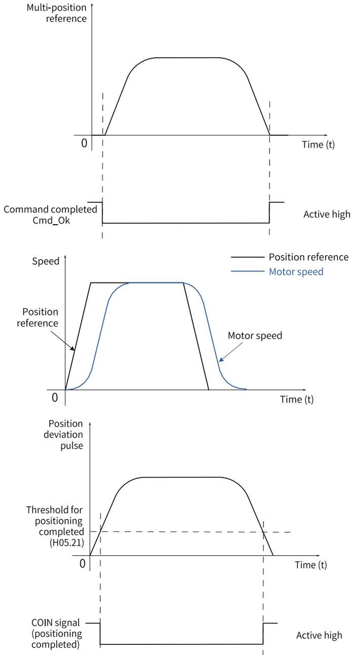
Figure 2-22 Description of positioning completed/proximity functions
