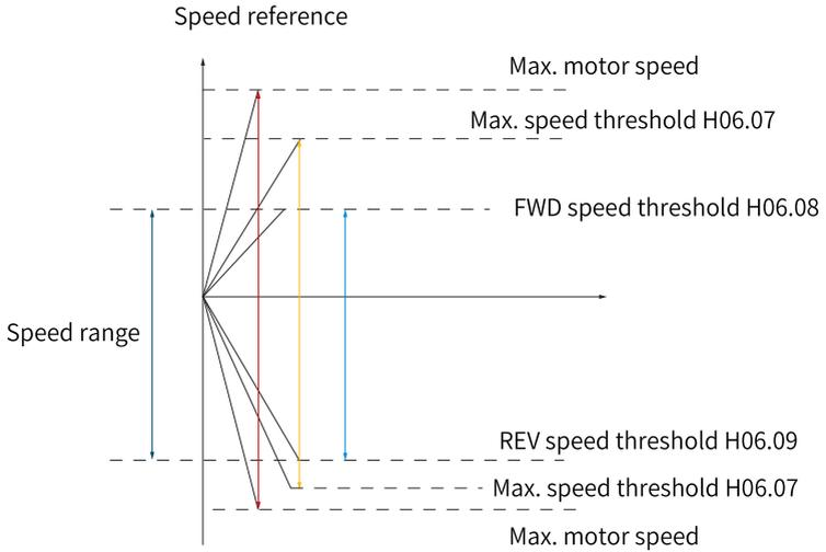
Figure 3-1 Example of speed reference limit
