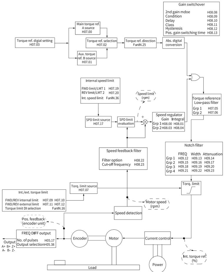
Figure 2-65 Block diagram of torque control parameters
