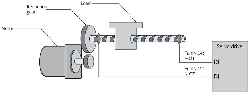
Figure 2-85 Installation of limit switches
