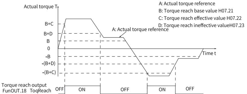
Figure 2-79 Example of TorReach signal waveform
