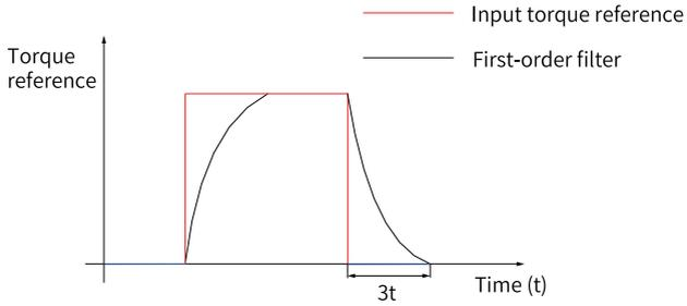
Figure 2-68 First-order filter for rectangular torque references
