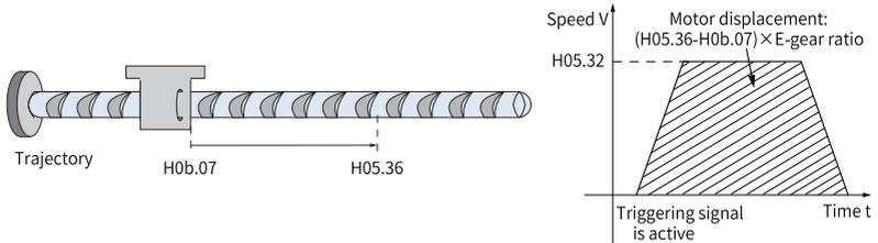
Figure 2-42 Motor running curve and speed in mode 14
