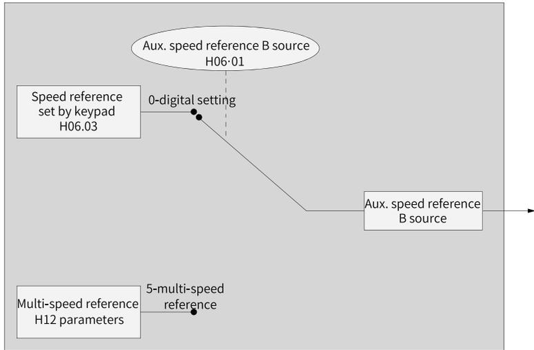
Figure 2-52 Source of auxiliary speed reference B
