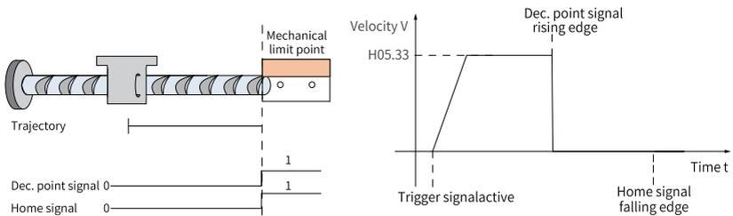
Figure 2-40 Motor running curve and speeds in Mode 10
