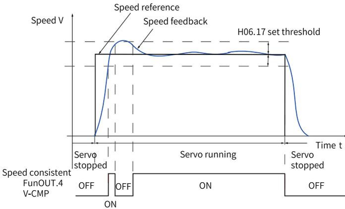
Figure 2-60 Waveform of speed matching (V-Cmp) signal
