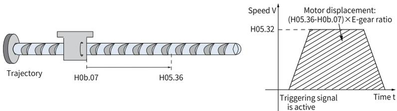
Figure 2-45 Motor running curve and speed in electrical homing
