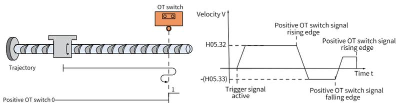
Figure 2-36 Motor running curve and speed in mode 6
