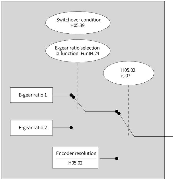
Figure 2-16 Procedure for setting the electronic gear ratio
