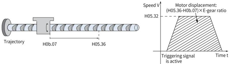
Figure 2-44 Motor running curve and speed in mode 16
