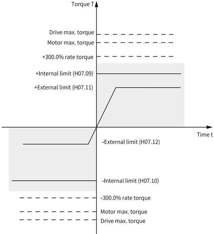
Figure 2-71 Example of torque limit
