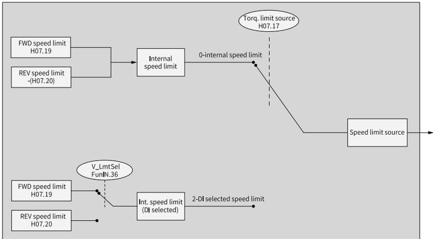
Figure 2-76 Speed limit source
