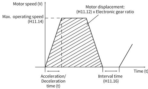
Figure 2-12 Motor operating curve in displacement 1
