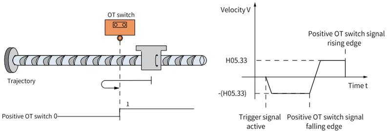
Figure 2-37 Motor running curve and speed in mode 6
