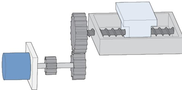
Figure 2-81 Ball screw transmission mechanism
