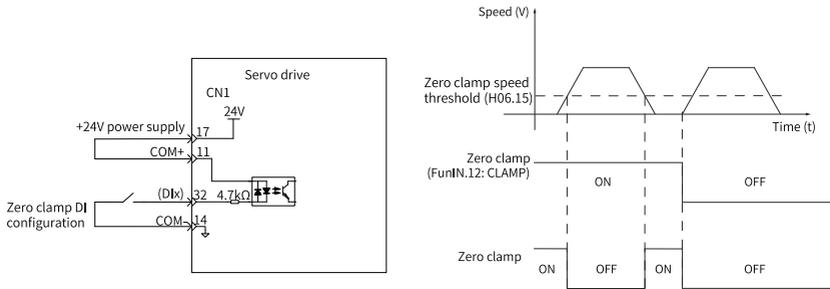
Figure 2-57 Wiring and waveform of zero clamp
