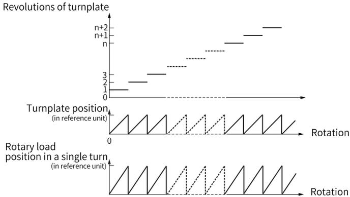
Figure 2-83 Relation between the single-turn position of the rotating load and the position of the rotating platform
