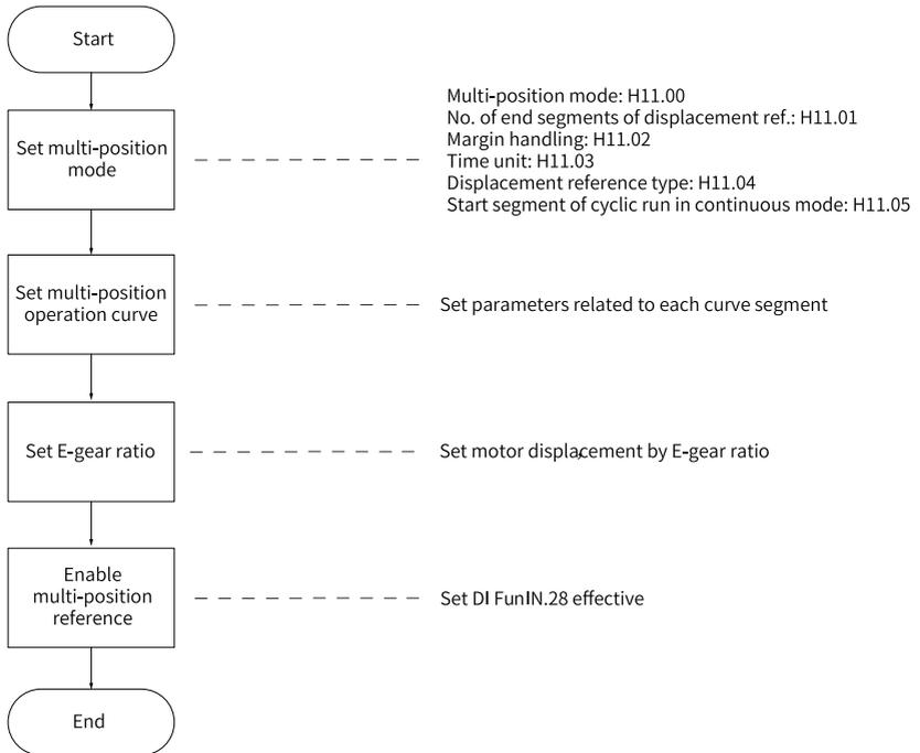
Figure 2-10 Flowchart for setting the multi-position reference as the source
