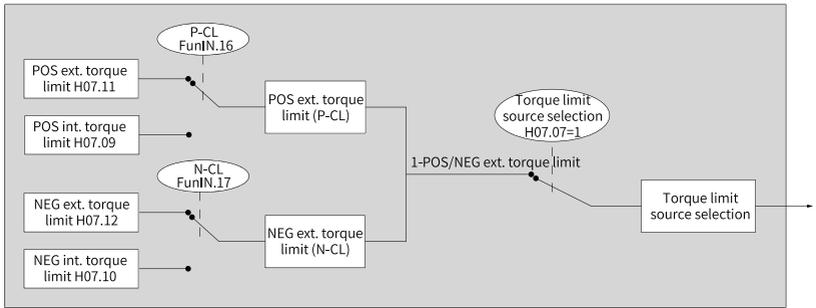
Figure 2-74 Torque limit source (H07.07 = 1)
