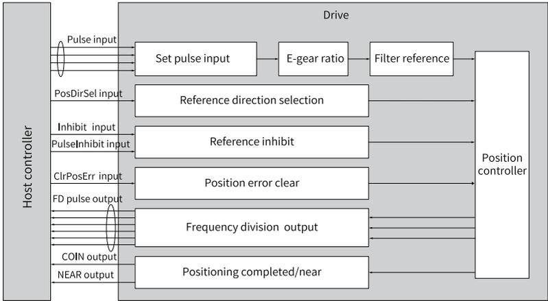
Figure 2-2 Signal exchange between the drive and the host controller
