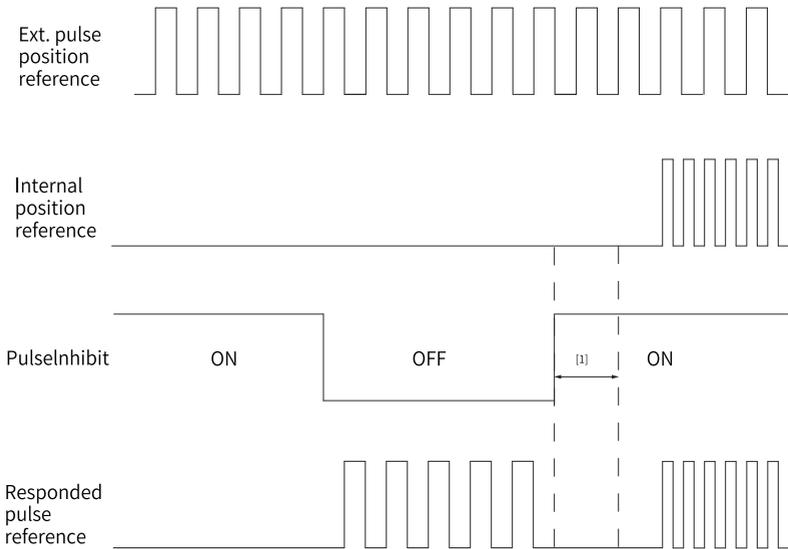
Figure 2-14 Waveform example for pulse reference inhibited
