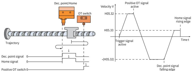
Figure 2-29 Motor running curve and speed in mode 0
