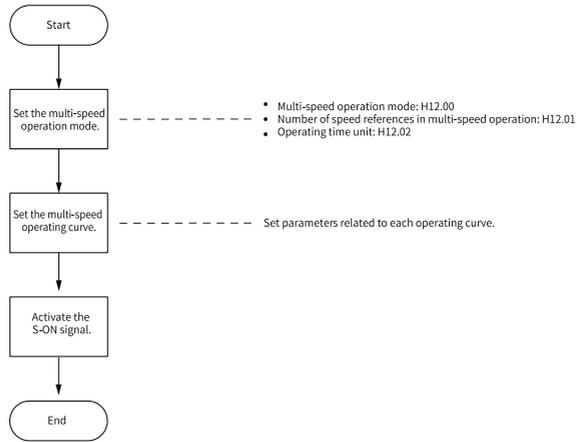
Figure 2-53 Flowchart for setting multi-speed operation
