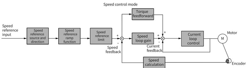
Figure 2-47 Block diagram of speed control
