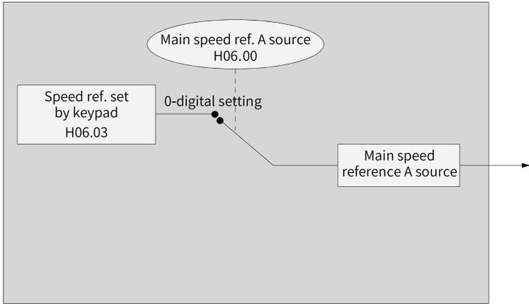
Figure 2-51 Source of main speed reference A
