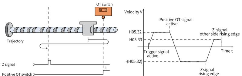
Figure 2-32 Motor running curve and speed in mode 2
