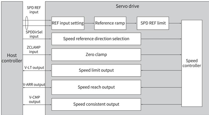
Figure 2-48 Signal exchange between the drive and the host controller
