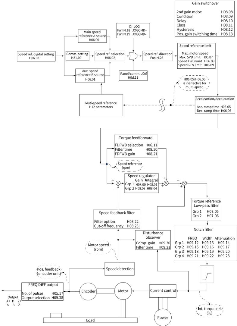
Figure 2-49 Block diagram of speed control parameters
