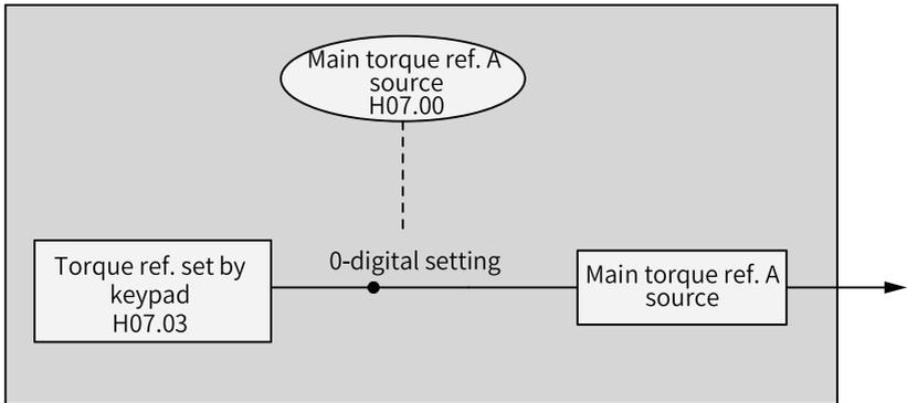
Figure 2-67 Description of source of main torque reference A
