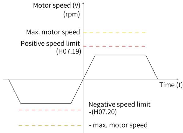
Figure 2-77 Speed limit curve (H07.17 = 0)
