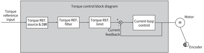
Figure 2-63 Block diagram of torque control mode
