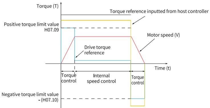
Figure 2-73 Torque limit curve (H07.07 = 0)
