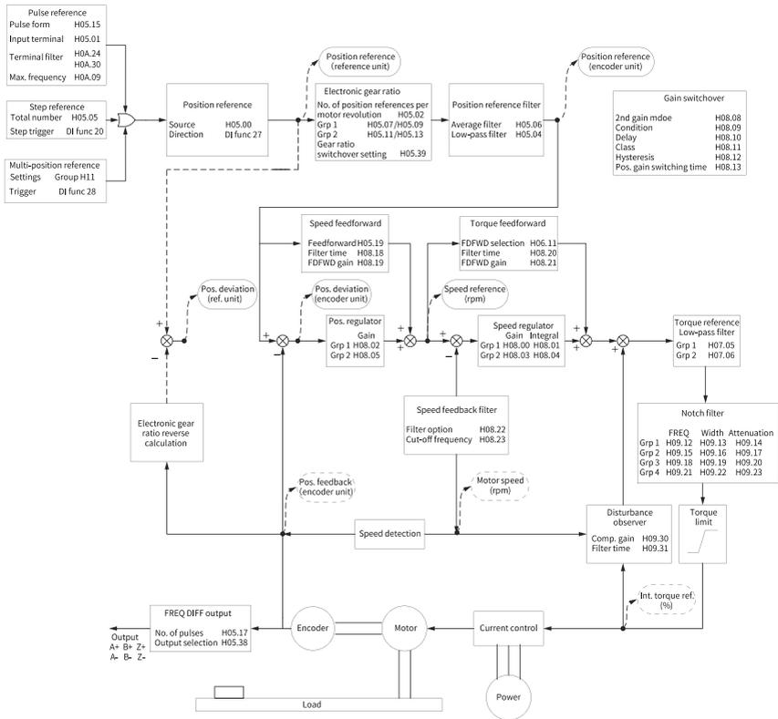
Figure 2-3 Block diagram of position control parameters
