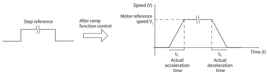
Figure 2-56 Ramp function definition
