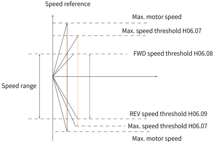
Figure 2-58 Example of speed reference limit
