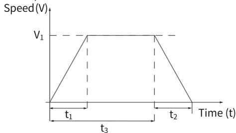
Figure 2-55 Example of multi-speed curve
