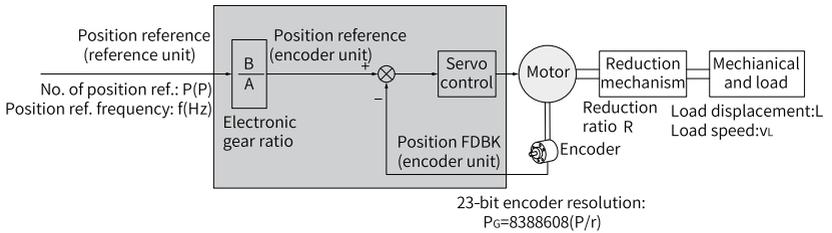
Figure 2-17 Relationship among the position reference (reference unit), load displacement, and electronic gear ratio
