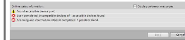
If the connection is normal, **Load** in the preceding figure will be available. You can click **Load** to start download and perform subsequent operations as prompted to download the configuration to the PLC.
