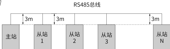
Figure 2-6 Branch line connection
