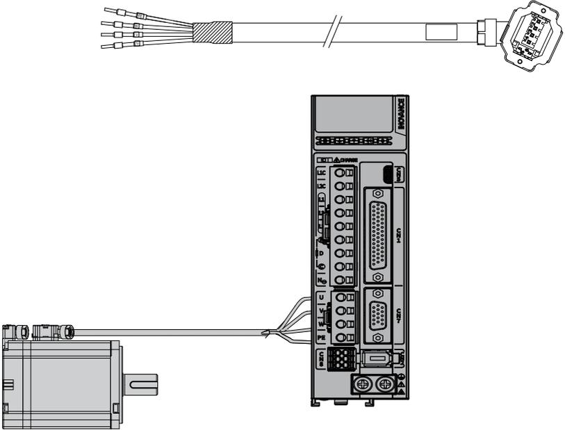
Figure 4-2 Wiring between the servo drive and terminal-type motor
