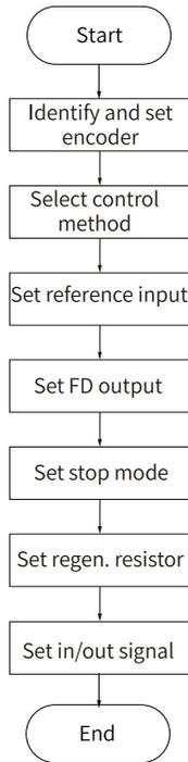
Figure 6-6 Setup wizard process
