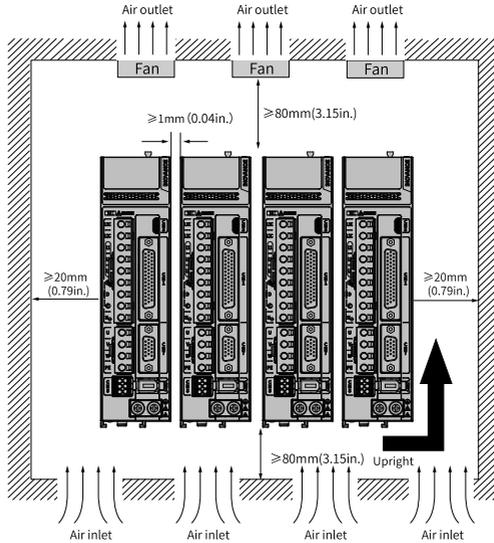
Figure 3-4 Clearance for compact installation
