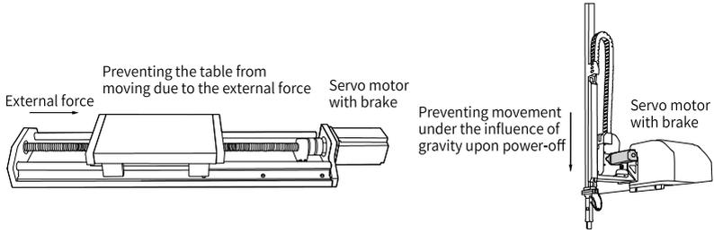
Figure 6-7 Application of the brake
