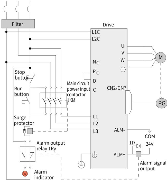
Figure 4-6 Main circuit wiring
