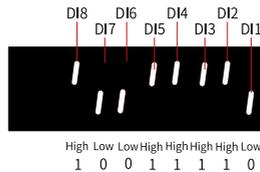
Figure 5-9 DI level states corresponding to bits of H0b.03
