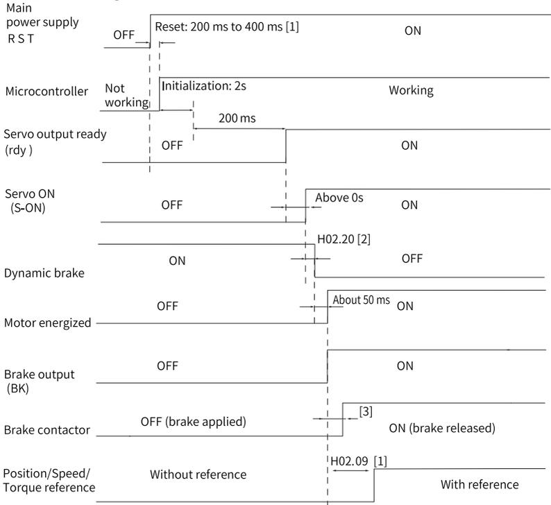
Figure 6-14 Power-on sequence diagram
