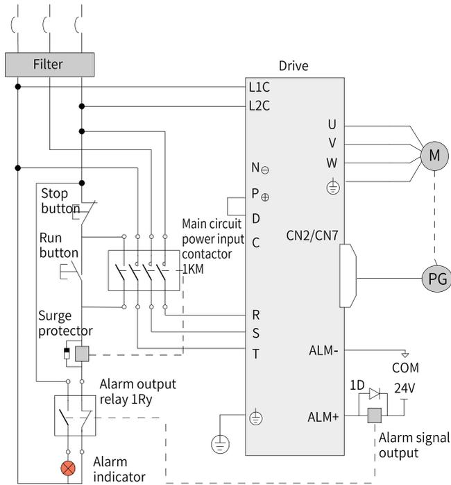
Figure 4-7 Main circuit wiring
