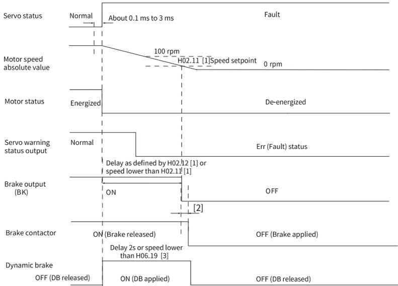
Figure 6-16 Sequence of "Dynamic braking stop, keeping de-energized state" at No. 1 fault
