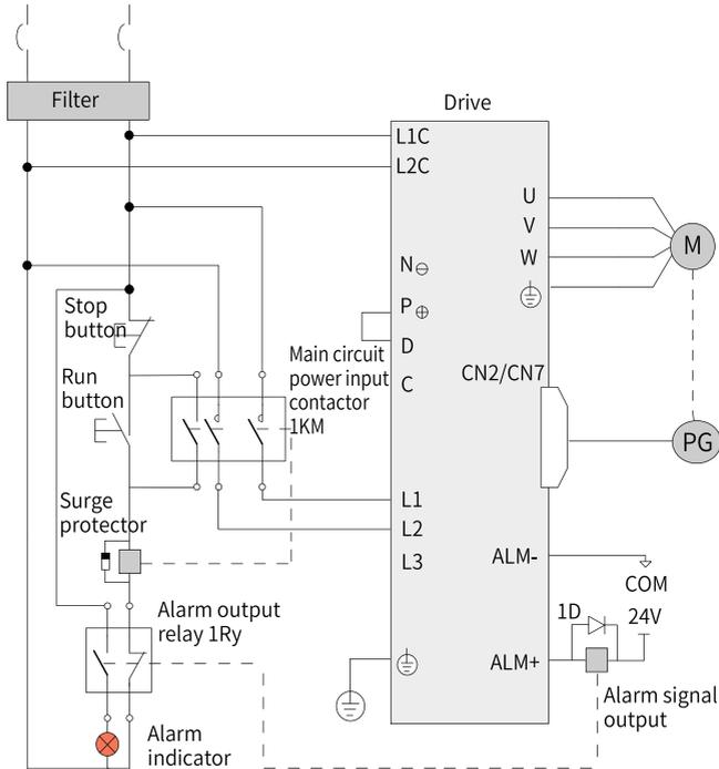
Figure 4-5 Main circuit wiring
