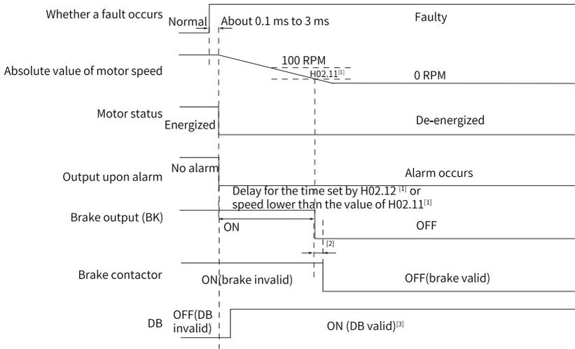
Figure 6-17 Sequence of "Dynamic braking stop, keeping dynamic braking state" at No. 1 fault
