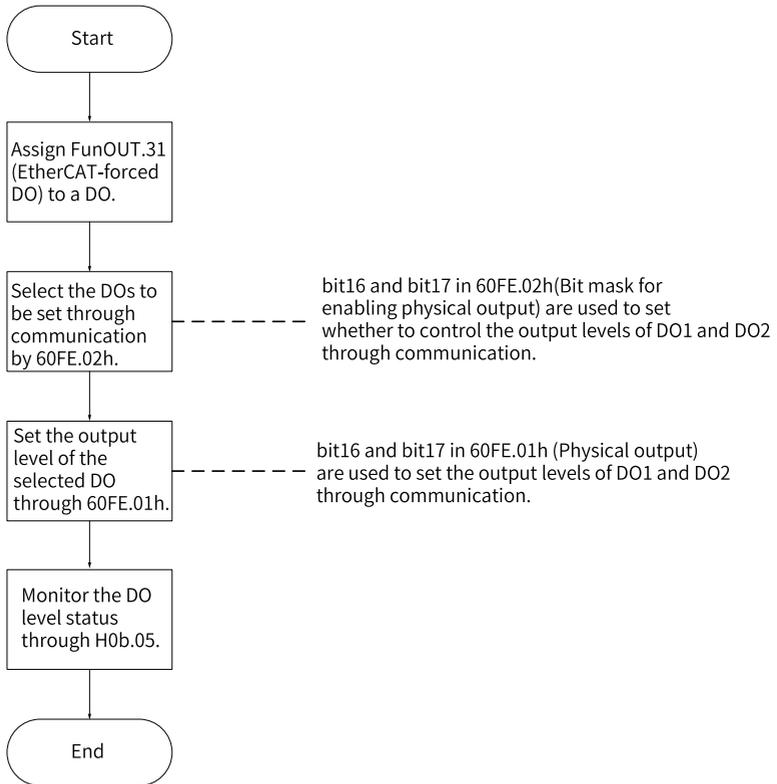
Figure 5-14 Procedure for setting forced DO function in bus control mode
