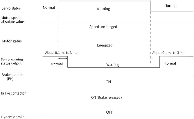
Figure 6-25 Sequence for alarms that do not cause stop
