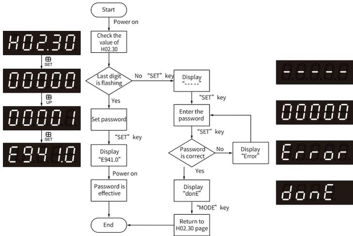
Figure 5-16 Procedure for setting the user password
