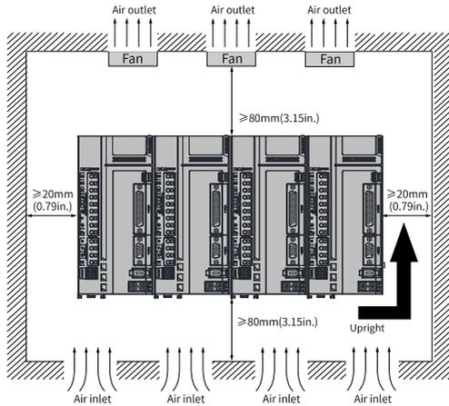
Figure 3-5 Zero-clearance installation
