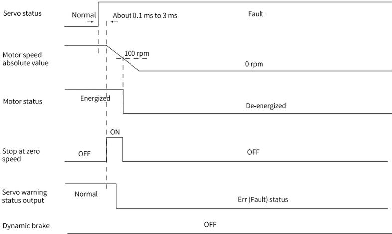
Figure 6-19 Sequence of "Stop at zero speed, keeping de-energized state" at No. 2 fault (without brake)
