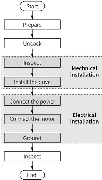
Figure 3-1 Installation flow chart
