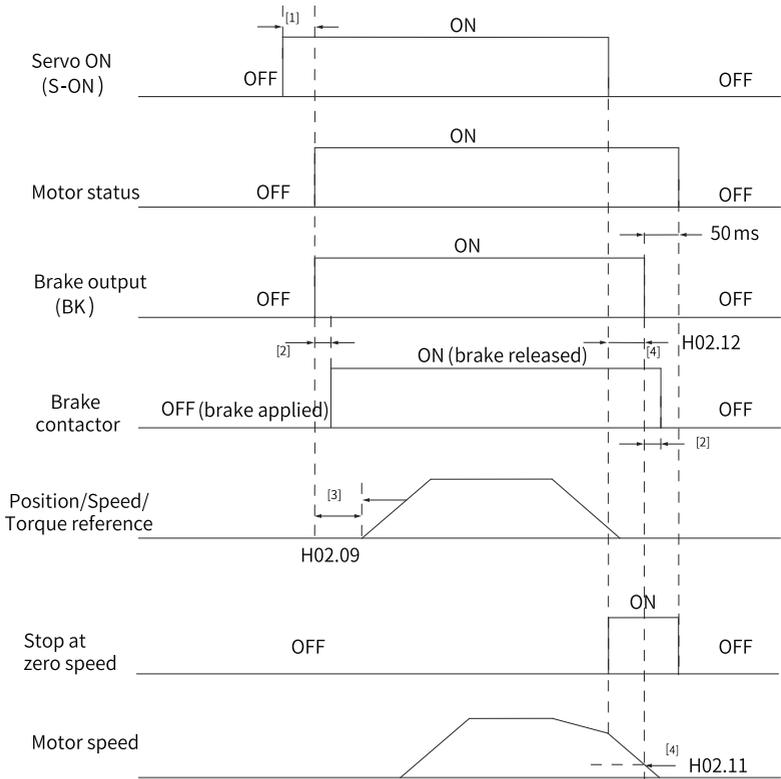
Figure 6-9 Brake sequence for a rotating motor
