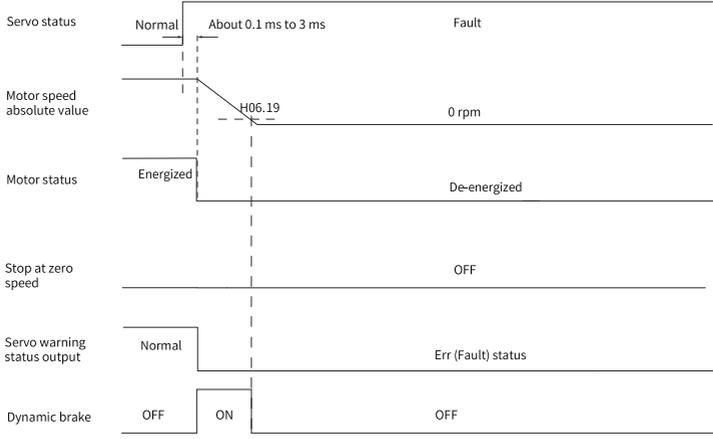
Figure 6-22 Sequence of "Dynamic braking stop, keeping de-energized state" at No. 2 fault (without brake)
