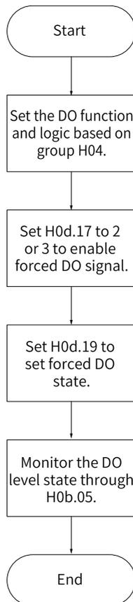
Figure 5-10 Procedure for setting forced DO function
