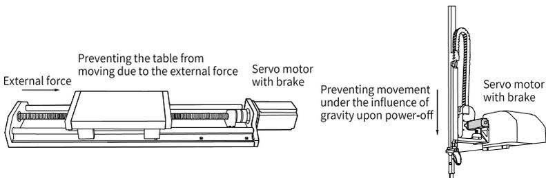
Figure 6-11 Application of the brake
