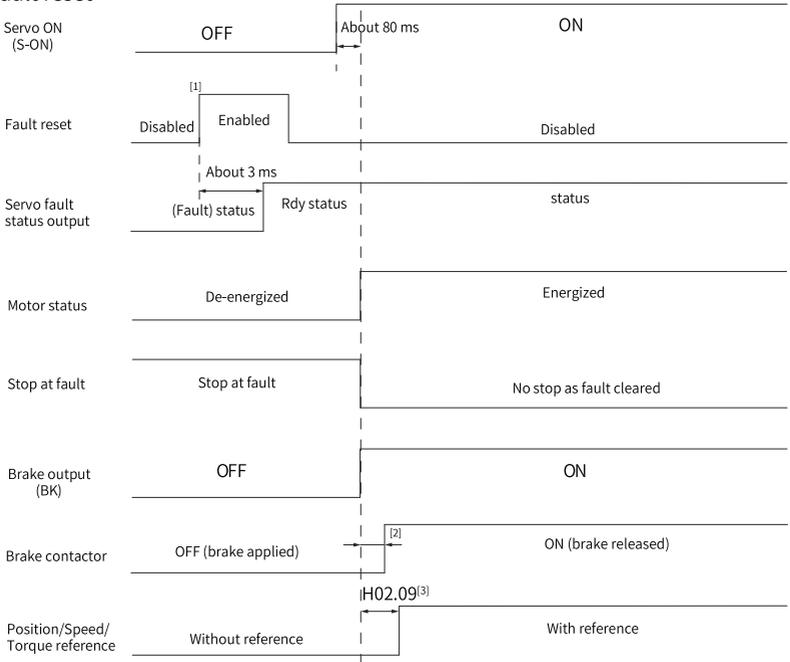
Figure 6-26 Sequence for fault reset
