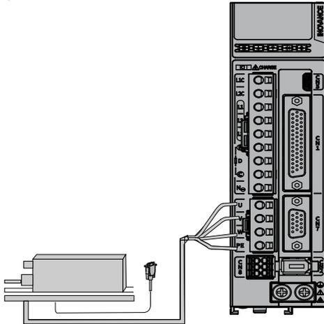
Figure 4-4 Wiring between the servo drive and DDL motor
