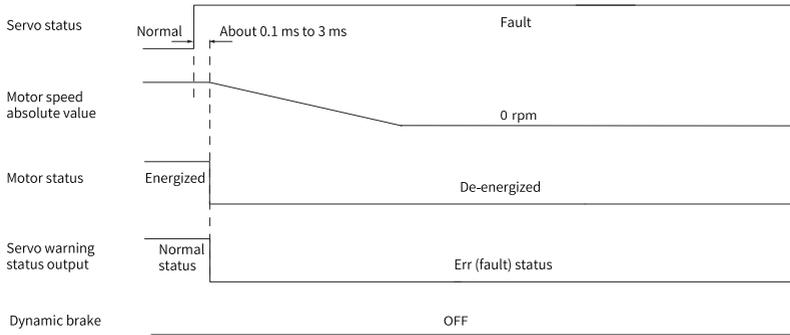
Figure 6-18 Sequence of "Coast to stop, keeping de-energized state" at No. 2 fault
