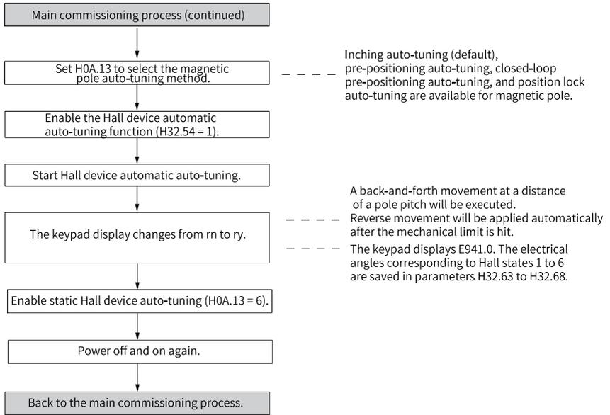
Figure 6-4 Flowchart for magnetic pole auto-tuning with a Hall device
