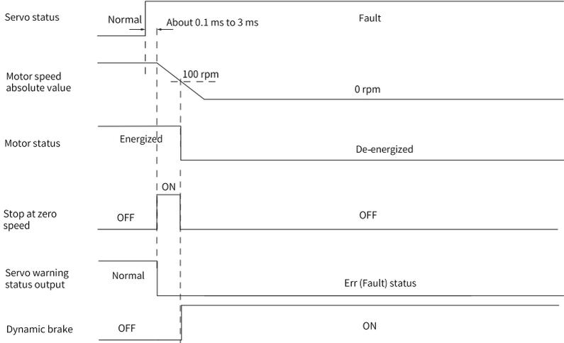
Figure 6-20 Sequence of "Stop at zero speed, keeping dynamic braking state" at No. 2 fault (without brake)
