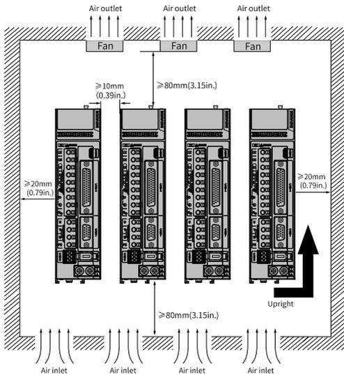
Figure 3-3 Clearance for side-by-side installation
