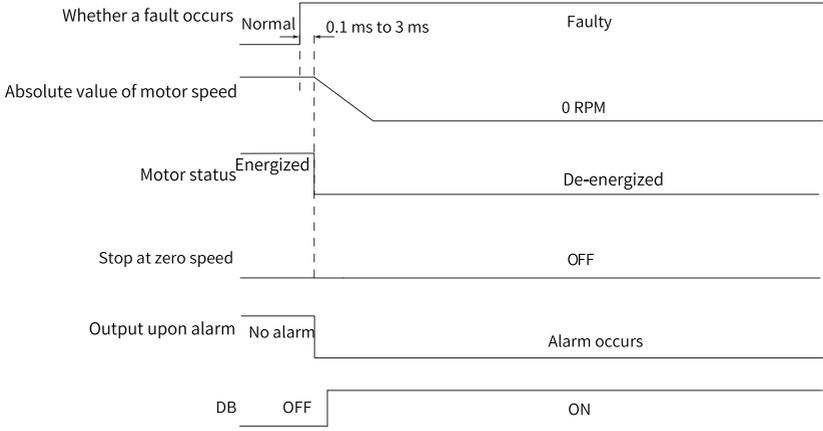
Figure 6-21 Sequence of "Dynamic braking stop, keeping dynamic braking state" at No. 2 fault (without brake)
