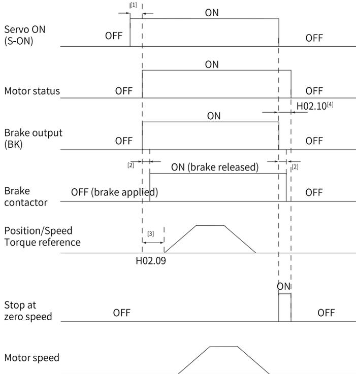
Figure 6-8 Brake sequence for motor at standstill
