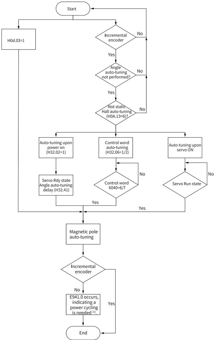
Figure 6-2 Flow chart of magnetic pole auto-tuning state
