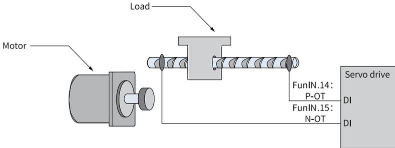
Figure 6-27 Installation of limit switches
