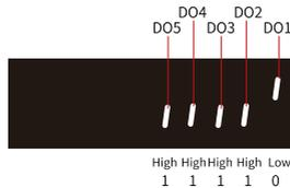
Figure 5-12 Display of H0b.05 when all DOs are active low
