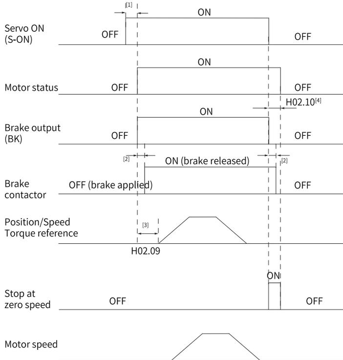
Figure 6-12 Brake time sequence for the motor in the static state
