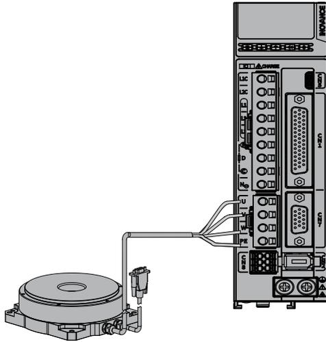
Figure 4-3 Wiring between the servo drive and DDR motor
