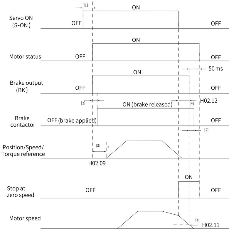
Figure 6-13 Brake time sequence for the motor in the rotation state
