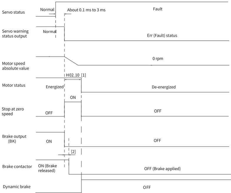
Figure 6-23 Sequence of "Stop at zero speed, keeping dynamic braking state" at No. 2 fault (with brake)
