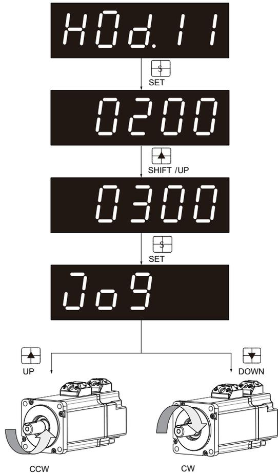
Figure 6-5 Procedure for setting the jog function
