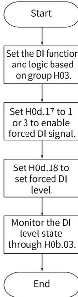
Figure 5-7 Procedure for setting forced DI function
