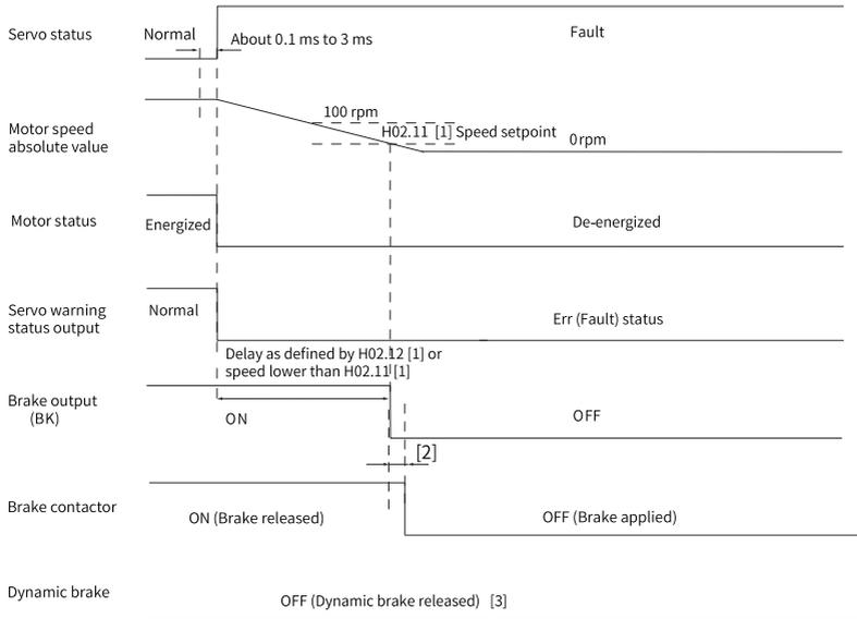
Figure 6-15 Sequence of "coast to stop, keeping de-energized state" at No. 1 fault
