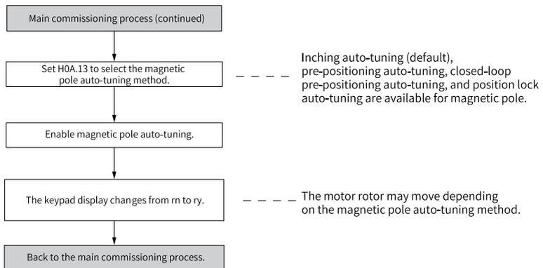
Figure 6-3 Flowchart for magnetic pole auto-tuning without a Hall device
