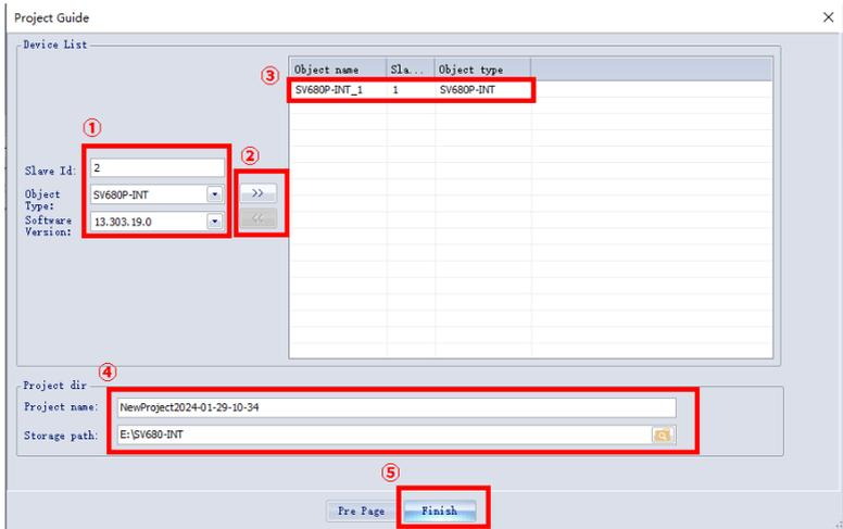
Figure 5-20 Project Guide interface for offline device
