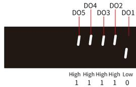
Figure 5-13 Display of H0b.05 when all DOs are active high
