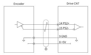
Suppose the current consumed by the motor encoder is 200 mA, you can select the cable based on the following recommendations.
