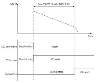
If the SS2 command is canceled after SS2 has been triggered, the SS2 state remains until the delay time has elapsed.
