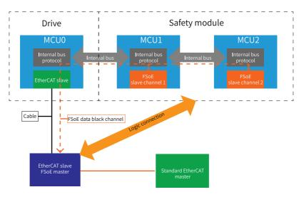
Figure 6-3 FSoE data transmission
