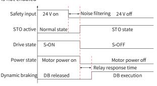
The safety module starts to shift to STO status when any of the STO inputs 1 and 2 is turned to "OFF".
