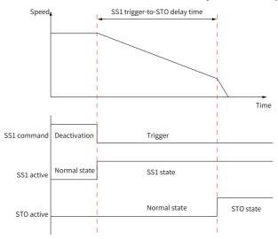
After SS1 is triggered, the SS1 command is canceled during the stop process of SS1. The drive continues to execute the stop process until the stop process is done.
