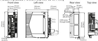
Figure 4-6 Dimension drawing of servo drives in size A
