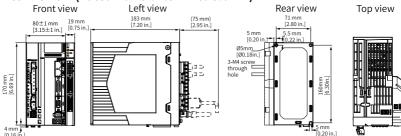
Figure 4-8 Dimension drawing of servo drives in size D
