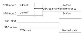
When an Ack signal is required, exiting the STO state not only needs the recovery of the 24V voltage, but also a trigger for an Ack signal. The S-ON operation can only be performed properly after STO state exits normally.
