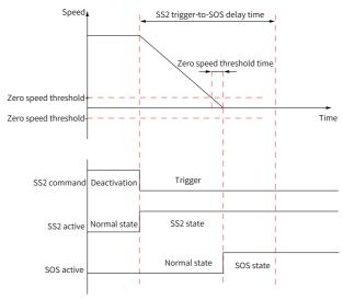
If the SS2 command is deselected after SS2 has been triggered, the SS2 state remains until the delay time has elapsed or the zero speed conditions are met.
