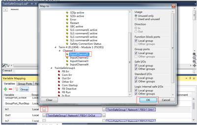
c. Set In2 to "InputChannel2", In3 to "InputChannel3", and In4 to "InputChannel4", respectively.
