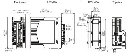
Figure 4-7 Dimension drawing of servo drives in size C
