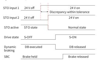
When the Ack signal is not required, the STO state can exit automatically as long as the 24 V DI input signal of two STOs are recovered. The S-ON operation can only be performed properly after STO state exits normally.
