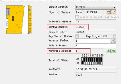
b. Check the serial number and hardware address of the EL6900 module.
