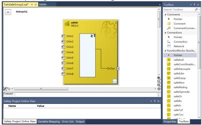
c. Four safety DI inputs are used to trigger the safety function. There are four safeOr
