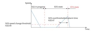
Figure 6-14 SOS speed change threshold
