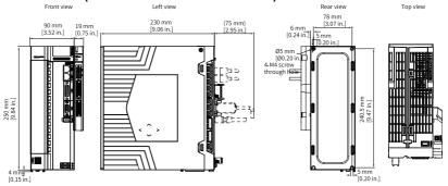
Figure 4-9 Dimension drawing of servo drives in size E
