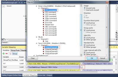
Use In1 to control the control word corresponding to STO and Out1 to indicate the state of In1.
