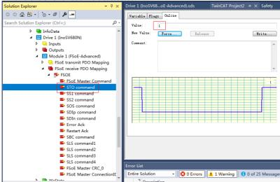
6. Disconnect the safety DI2. The bit in RPDO corresponding to SS1 command changes to "0" and the SS1 function is triggered.
