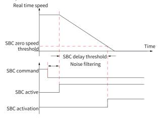
Figure 6-5 Response sequence of SBC execution
