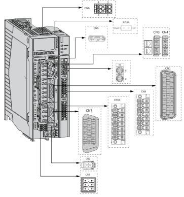
Figure 5-1 Terminal pin layout of the servo drive
