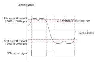
The purpose of the SSM hysteresis setting is to achieve a stable signal output when the motor speed is near the upper and lower SSM threshold. The SSM function prevents the SSM output signal from jumping back and forth between 0 and 1 several times around the threshold due to the real-time fluctuation of the motor speed.
