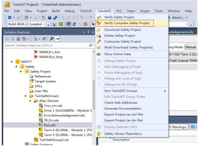
b. After verification is complete, check whether there is an error and whether the message "Verification Process succeeded" appears in the lower left corner. The
