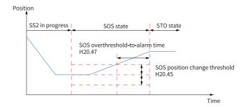
Figure 6-15 SOS position change threshold
