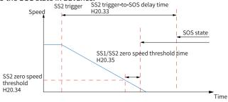
Figure 6-11 Safety function triggered by the local mode, motor speed changing
