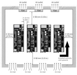
Figure 4-3 Clearance for side-by-side installation
