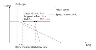
Figure 6-9 Motor speed when ramp limit is triggered
