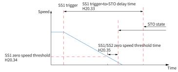
Figure 6-7 Safety function triggered by the local mode, motor speed changing
