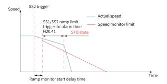
Figure 6-13 Motor speed when ramp limit is triggered
