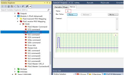
Restore the safety DI2. The bit in RPDO corresponding to SS1 command changes to
