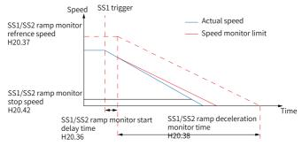
Figure 6-8 Motor speed when safety function is triggered
