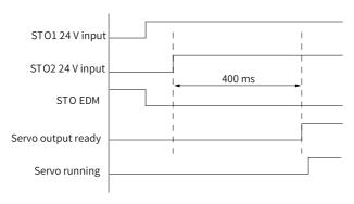
Figure 7-3 Servo drive reset sequence diagram
