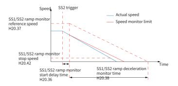
Figure 6-12 Motor speed when safety function is triggered
