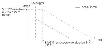
Figure 6-10 Motor speed during ramp-to-stop
