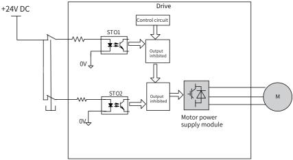
Motor-torque-off is achieved by cutting off the motor supply current through cutting off motor power supply module output.
