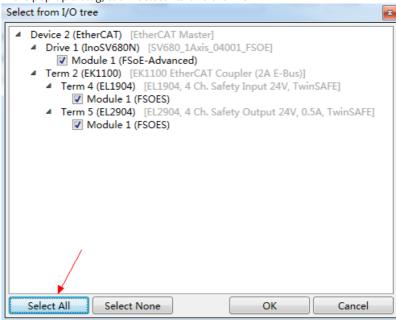
c. Add safety I/O module and safety module under "Alias Devices".
