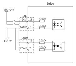
The safety DI is a sink-type input. Perform wiring according to the characteristics of the load circuit.
