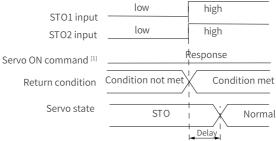
Figure 7-2 Return condition of external STO request state
