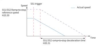
Figure 6-6 Motor speed during ramp-to-stop
