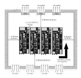
Figure 4-4 Clearance for compact installation
