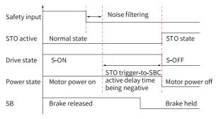
When SBC is activated before STO and the STO input command is active, the stop mode defined by H02.05 is executed first. When the delay defined by H20.28 elapses, the stop mode defined by H02.08 is triggered then.
