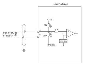
Figure 5-4 PTC wiring diagram
