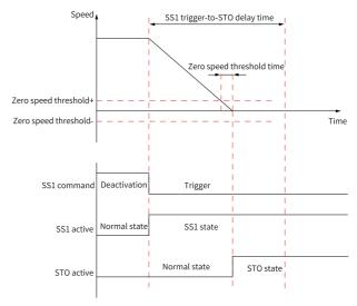
If the SS1 command is canceled after SS1 has been triggered, the SS1 stop state still remains until the delay time has elapsed or the zero speed conditions are met.
