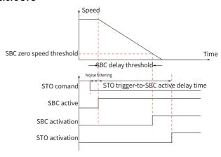
When the delay H20.28 from STO activation to SBC activation is negative, the servo drive performs deceleration after the safety module receives the STO trigger command.
