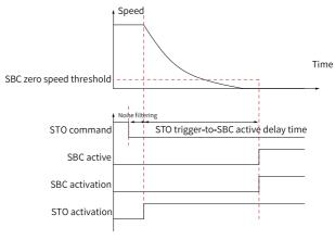
When the delay H20.28 from STO activation to SBC activation is positive, after the safety module receives the STO trigger command, the drive cuts off the S-ON signal and performs coast-to-stop, and triggers the SBC function when the delay is reached.
