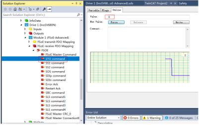
Restore the safety DI1. The bit in RPDO corresponding to STO command changes to
