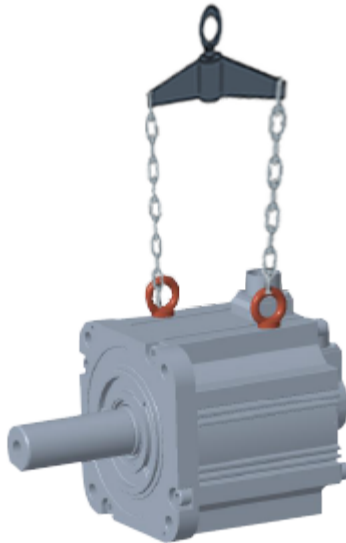
Figure 4-2 Hoisting and handling the motor through the eyebolt
