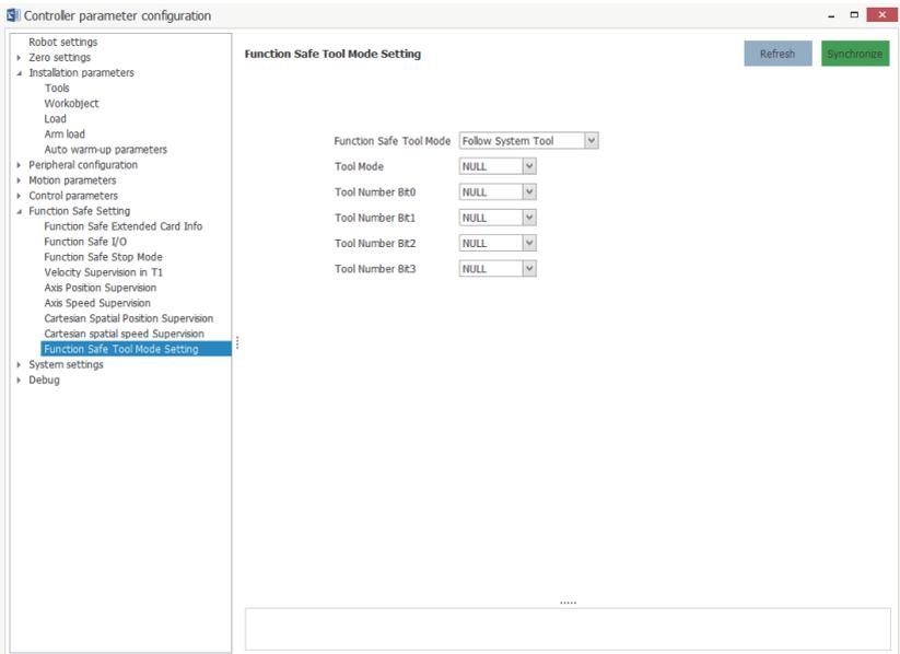
2. If you set the safety tool to fixed safety tool, you need to specify a tool (TCP mode) or a workobject (ECP mode) as the safety tool\workobject. In this case, you cannot switch the safety tool via safety I/O or standard I/O. The selected workobject must be held by the robot.
