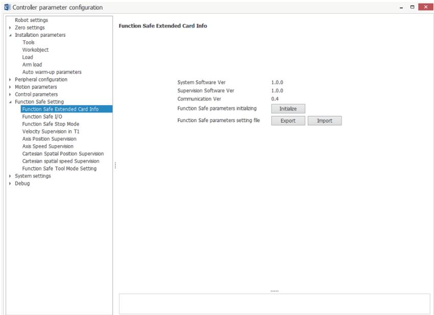
After the safety parameters are initialized, the parameters saved in the safety expansion card will be restored to the factory settings. Use this function with caution.
