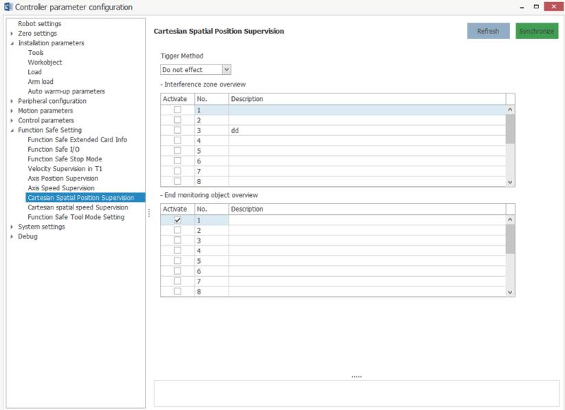
6. Check the interference zone and monitoring object to be used.
