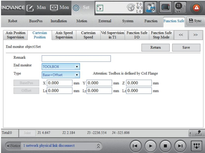
When the point acquisition method is set to "base point + offset", you can enter the base point and the offset manually, or click the **Base point** button to get the point automatically and then manually enter the offset. Note that the **Base point** button takes effect only when the robot is in ECP mode. The point and offset are taken in the flange coordinate system. The range of the point value is [-10000,10000], and the range of the offset is [-10000,0), (0,10000], in mm.
