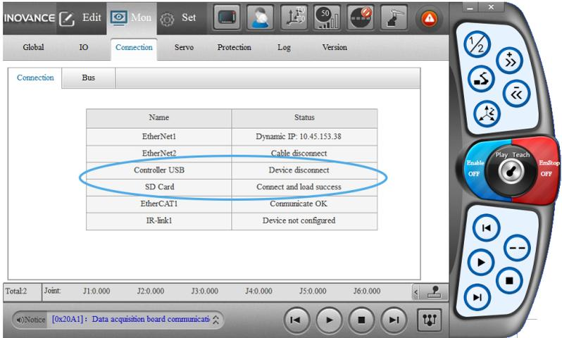
2. Click the backup button and confirm. The system backs up the program automatically and exits when the loading is complete.
