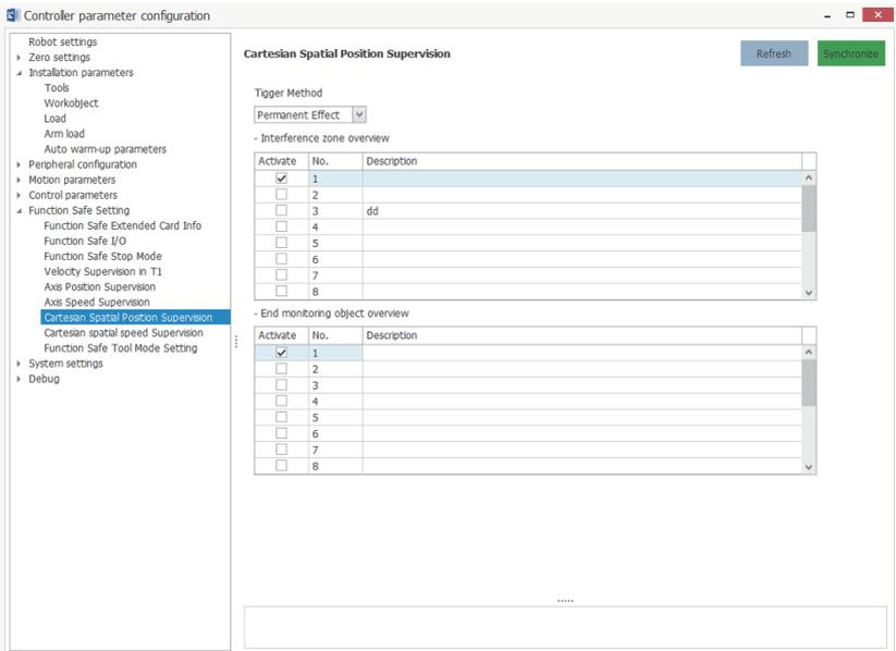
After the parameters are configured and saved, the TCP position monitoring function takes effect immediately.
