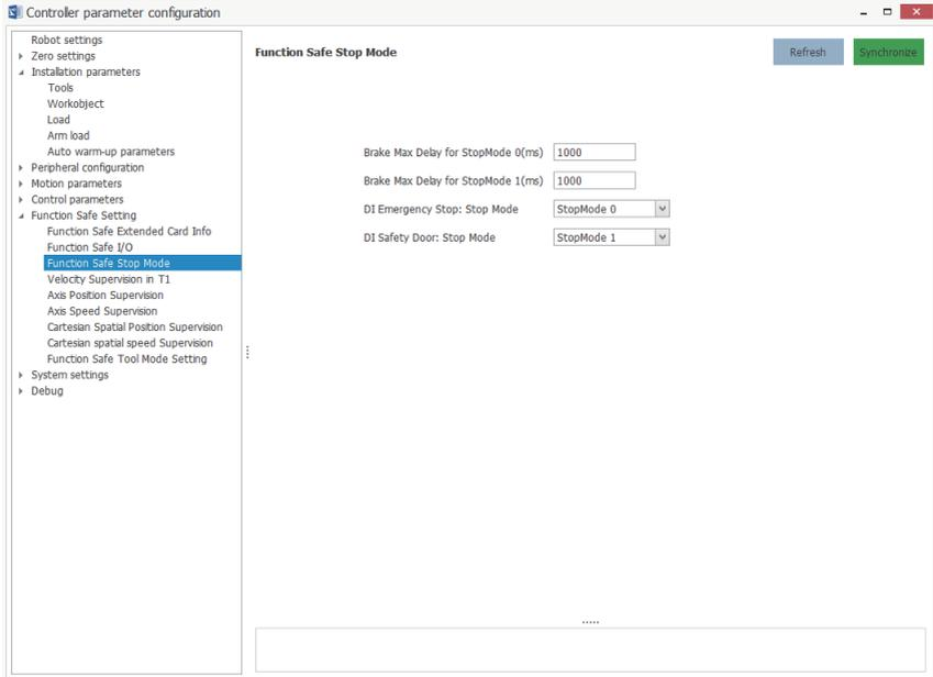
The safety stop parameters take effect immediately after being configured and saved.
