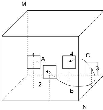
1 and 4 are located within the safety zone, while 2 and 3 are located on the critical plane of safety zone; trajectory segments A and C are located within the safety zone, while B is located outside the safety zone.
