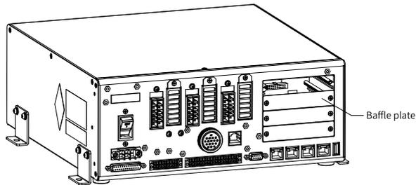
2. Align the expansion card with and insert it into the card slot and then tighten the expansion card with the Phillips screwdriver.
