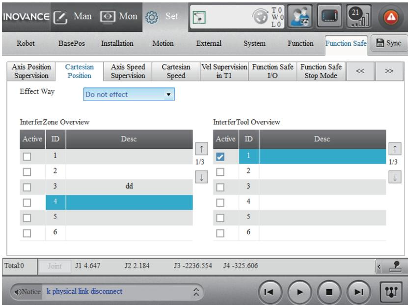
8. Check the interference zone and monitoring object to be used.
