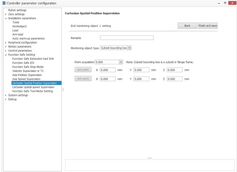
When the point acquisition method is set to "diagonal point", you can enter the point manually or click the **Get point** button to acquire the current point automatically. Note that the **Get point** button is active only when the robot is in ECP mode. The points are taken in the flange coordinate system. The range of the point value is [-10000,10000], in mm.
