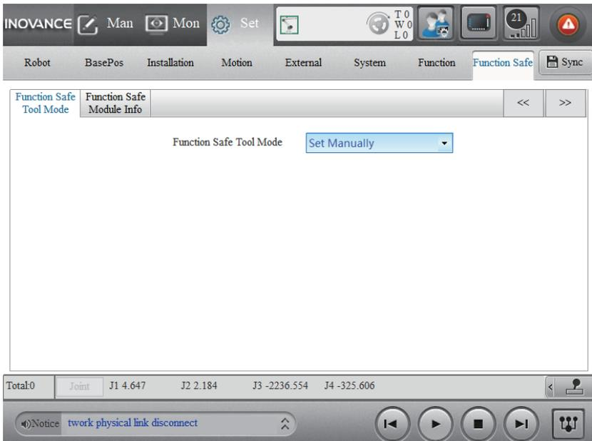
After the parameters are configured and saved, the safety tool set takes effect immediately.
