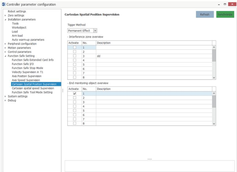
4. Select an end monitoring object and double-click it to open the parameter setting interface.
