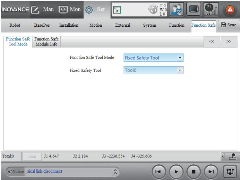
3. If you choose to manually switch the tool, you need to connect the external I/Os to the DI3-DI7 of the safety expansion card. The tool can be switched by the operator manually or by the external device.
