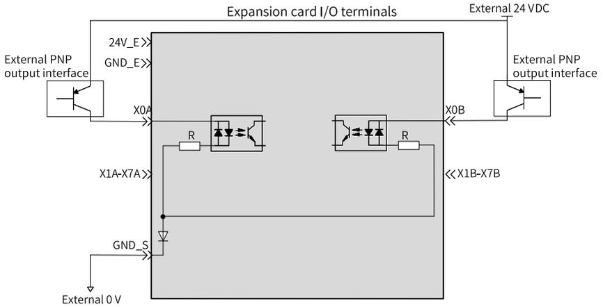
If an external 24 V power supply is used to power DI and the DO function is not needed, then 24V\_E and GND\_E can be connected or not. If the DO function is needed, it is necessary to perform wiring according to the DO wiring instructions.
